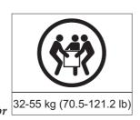
The weight of this part or unit is between 32 and 55 kg (70.5 and 121.2 lb). It takes three persons to safely lift this part or unit. (C010)
