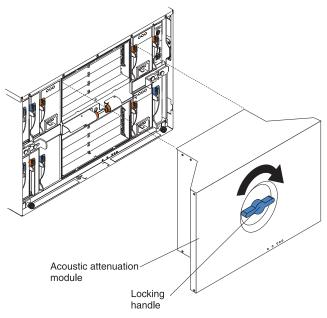
To install an acoustic attenuation module on the BladeCenter unit, complete the following steps:
