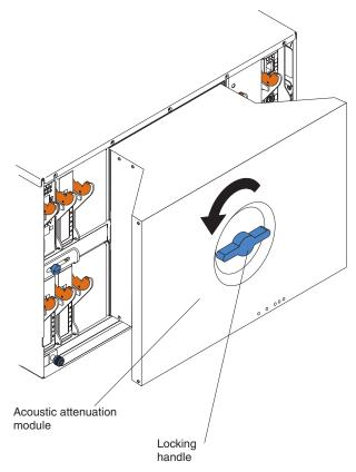
To remove an acoustic attenuation module from the BladeCenter unit, complete the following steps:
