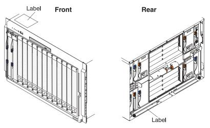
A set of blank labels comes with each blade server. Record all identifying information on a label and place it on the BladeCenter bezel, just below the blade server, as shown in the following illustration. Do not place the label on the blade server itself or in any way block the ventilation holes on the blade server.
