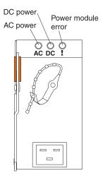
Power module LEDs: These LEDs indicate the condition of the power module.
