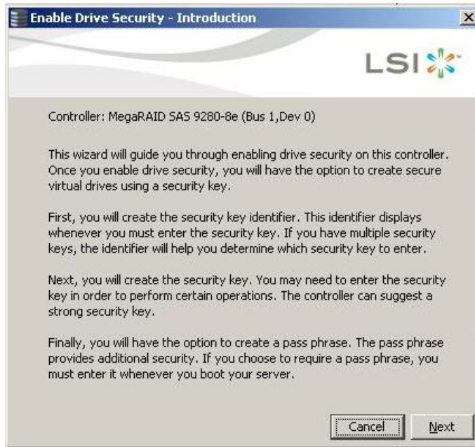
Figure 7.16 Enable Drive Security - Introduction Screen
