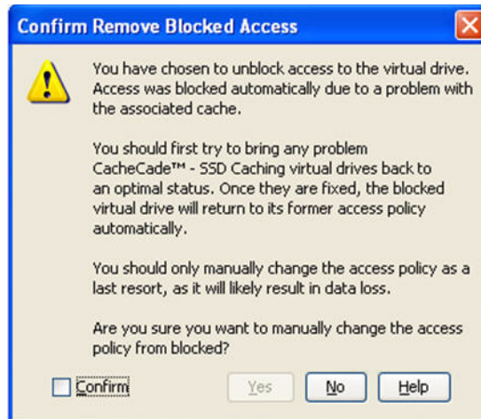
Figure 10.15 Confirm Remove Blocked Access
