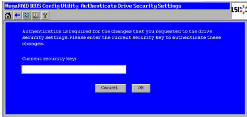
Figure 4.38 Authenticate Drive Security Key
