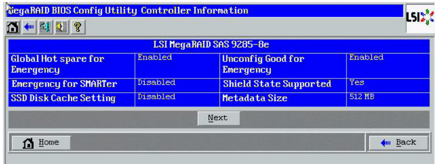
Figure 4.64 SSD Disk Cache Setting in Controller Properties Dialog
