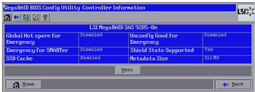
Figure 4.44 Second Controller Properties Screen
