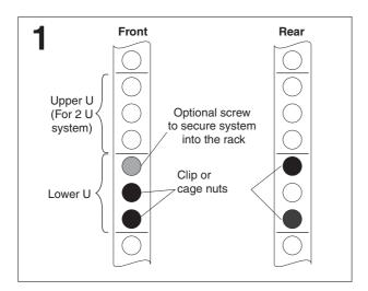
Select an available 1 U or 2 U space (depending on the server you are installing) in your rack to install your server. If you have either a round-holed or square-holed rack, install cage bars or clip nuts in the middle and the bottom (optional for the upper) holes of the lower U on each side of the front of the rack. Then, install cage bars or clip nuts in the upper and the bottom holes of the lower U on each side of the rear of the rack.
