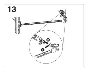
To attach the other side of the support arm to the backside of the slide rail, pull the pin out 1, and then slide the bracket 2 into the slide rail.
