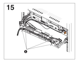
server (including keyboard, monitor, and mouse cables, if required). Route the cables and power cords on the cable-management arm 1 and secure them with cable ties or hook-and-loop fasteners.
