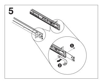
remove the bracket 2 from the rear of the slide rail.
