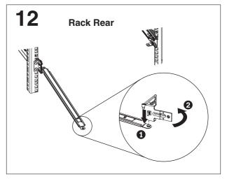
Install the L-shaped cable-management arm stop bracket 1 on the unattached end of the support arm. Turn the bracket 2 to secure it to the support arm.
