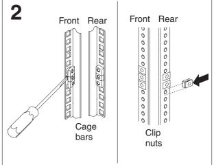
Use a screwdriver to install the cage bars or the clip nuts on the inside of the mounting rail, as required for your rack, into the selected holes.
