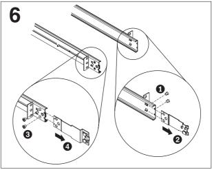
To remove the support bracket, remove the screw 1 and To remove the mounting brackets, remove the screws 1 and 3 . Slide out the brackets 2 and 4 from the rear of the slide rail. If you are installing the cable management arm on the right side then reinstall these brackets on the opposite slide rails to accommodate mounting of the cable management arm.
