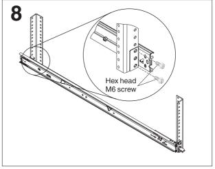
Use two screws to attach the rear of the slide rail to the rear of the rack cabinet in the upper and the bottom holes of the lower U.
