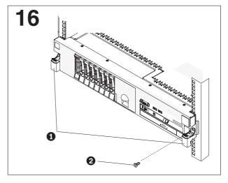
Attach the power cords and other cables to the rear of the Slide the server into the rack until it snaps into place. To slide the server out of the rack, press on the release latches 1
