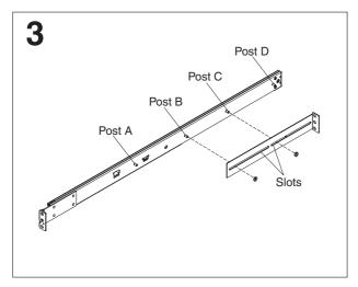
The rail depth can be adjusted from 17" (432 mm) to 31.25" (794 mm). To adjust the depth, you can loosen the nuts on the posts and slide the bracket until the distance between the front and rear slide rail flanges matches the distance between the front and rear EIA rails of the rack cabinet. If you need further adjustment, remove the nuts, move the bracket to the appropriate set of posts (A, B, C, and D) to obtain the appropriate slide rail depth, then reinstall and tighten the nuts.
