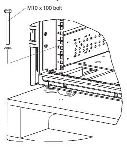
6. Open the rear doors and use the provided wrench to remove the two corner bolts that secure the rear of the rack to the pallet.
