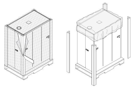
2. Remove the corner protectors and any other packaging material along with the plastic bag that covers the rack.
