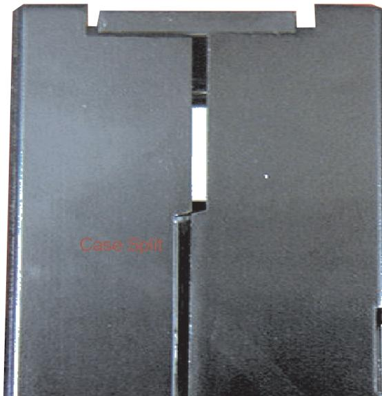
Figure 6. Checking for gaps in the seams of a cartridge
