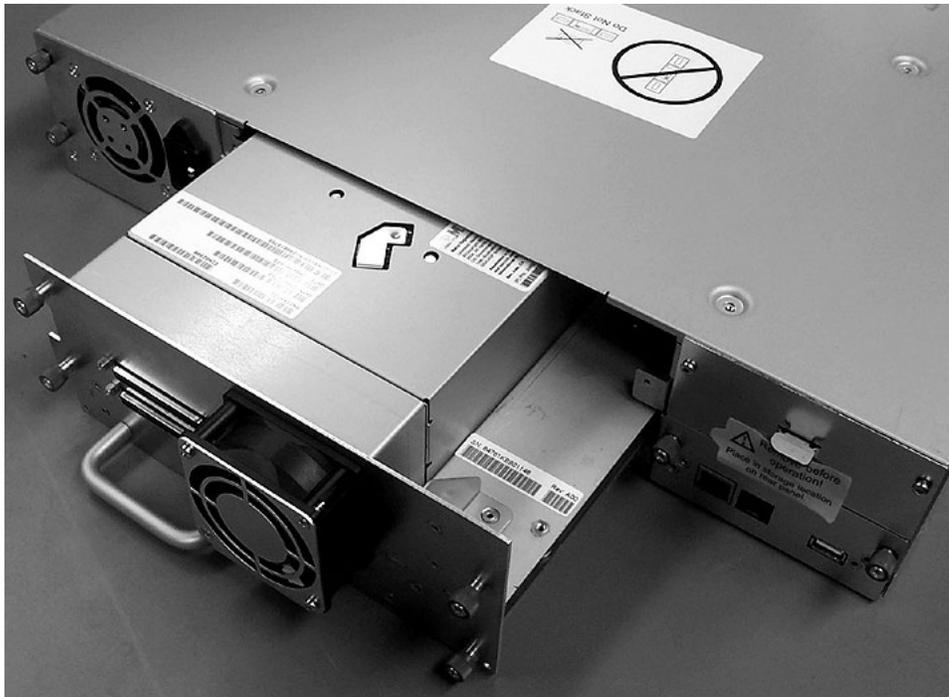
Figure 9. Removing the tape drive
