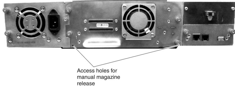
3. Push the end of a straightened paper clip (or a similar tool) into the access hole for the magazine that you want to remove.
