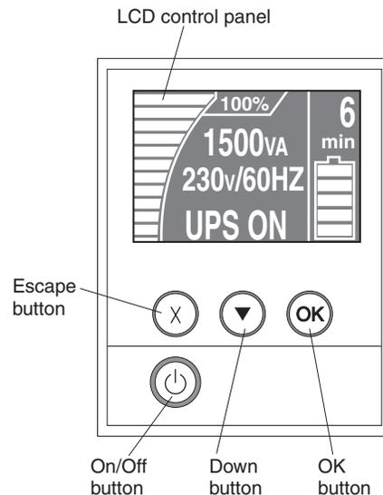
The uninterruptible power supply has a graphical liquid crystal display (LCD) with dual color backlight. Standard backlight is used to light the display with white text and a blue background. The display flashes if any alarms are active.
