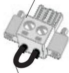
Remove jumper if installed
