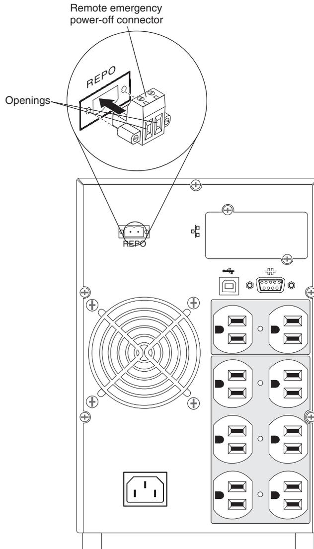
4. Connect the switch or circuit to the remote emergency power-off connector on the rear of the uninterruptible power supply using insulated size 18 - 20 AWG (0.75 mm<sup>2</sup> - 0.5 mm<sup>2</sup>) wire.
