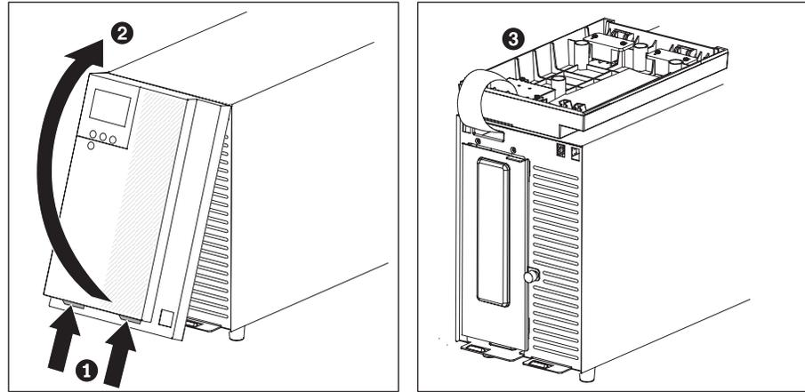
**Note:** A ribbon cable connects the front bezel to the uninterruptible power supply. Do not pull on the cable or disconnect it.
