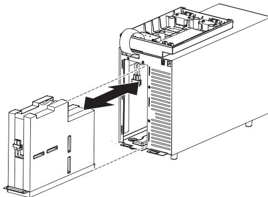
5. Carefully slide the new internal battery all the way into the battery bay.
