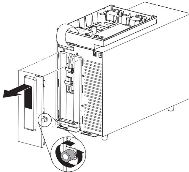
3. Disconnect the internal battery connectors.
