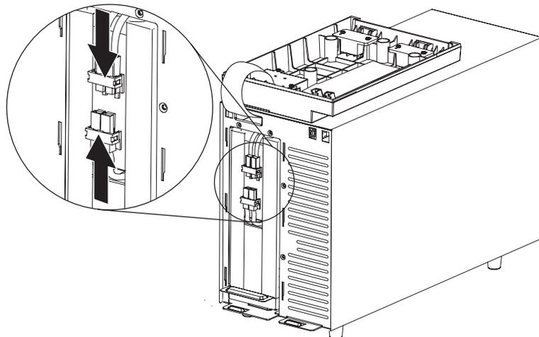
**Note:** A small amount of arcing might occur when you connect the batteries. This is normal and does not damage the unit or present any safety concern.
