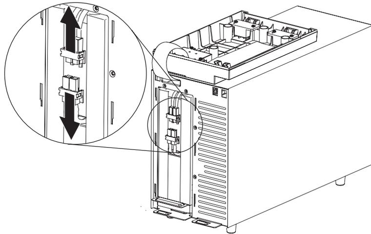
4. Grasp the plastic holder on the battery and carefully slide the battery module out of the uninterruptible power supply. Recycle the battery according to local ordinances.
