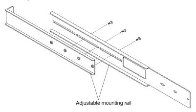
b. Secure the two adjustable mounting rail parts with three screws that come with the rack-mounting kit.
