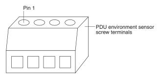
**Note:** External contact device 1 is connected between pins 1 and 2. Device 2 is connected between pins 3 and 4 (as labeled to show device 1 and 2). External contact devices can be normally open or normally closed.
