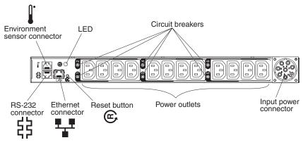
The following illustration shows the components and controls on the front of the 1U PDU with 9 C19 outlets on the front.
