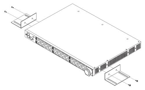
2. Hold the PDU in the side of the rack cabinet, and attach the vertical mounting brackets to the side braces with four M6 screws and nuts that come with the PDU.
