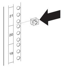
To install the PDU in the 1U mounting space in the side of an IBM Enterprise rack cabinet, complete the following steps:
