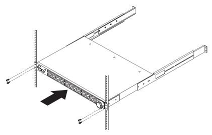
6. Secure the adjustable mounting rails and the 1U blank filler panel to the rack cabinet.
