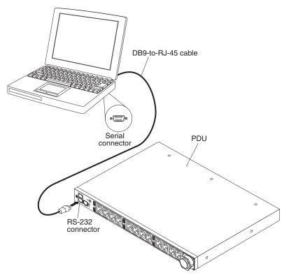
If your workstation or notebook computer does not have a DB9 serial connector, you can use a DB9-to-USB converter cable to connect the PDU to a workstation or notebook computer.
