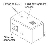
The PDU environment sensor kit comes with one PDU environment sensor, screws, hook-and-loop fasteners, and Ethernet cable. You can install the device anywhere on the rack by using either the screw or the self-adhesive hook-and-loop fasteners.
