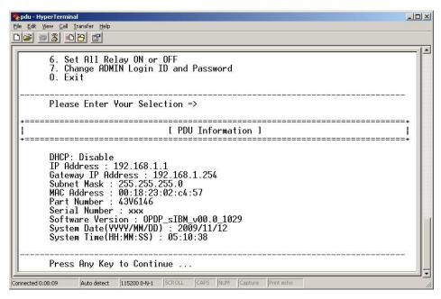
10. Press any key to return to the main menu. You can continue to use the PDU Configuration Utility, or you can use the Web interface to configure and monitor the PDU remotely. For more information, see "Using the Web interface" on page 31.
