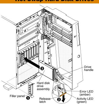
cotta on a component indicates that the component can be hot-swapped. Hot-swap means that if the system, operating system, and configuration all support hot-swap capability, you can remove or install the component while the system is running.
