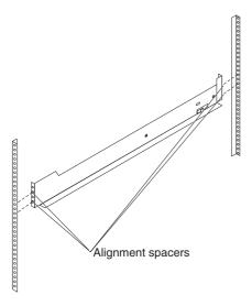
6. Secure the rail to the front of the rack cabinet with one M5 screw in the top hole of the bracket. For racks with square holes, add one washer between the M5 screw and the rail bracket.
