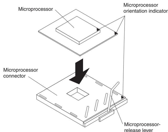
3. Close the microprocessor-release lever to secure the microprocessor.
