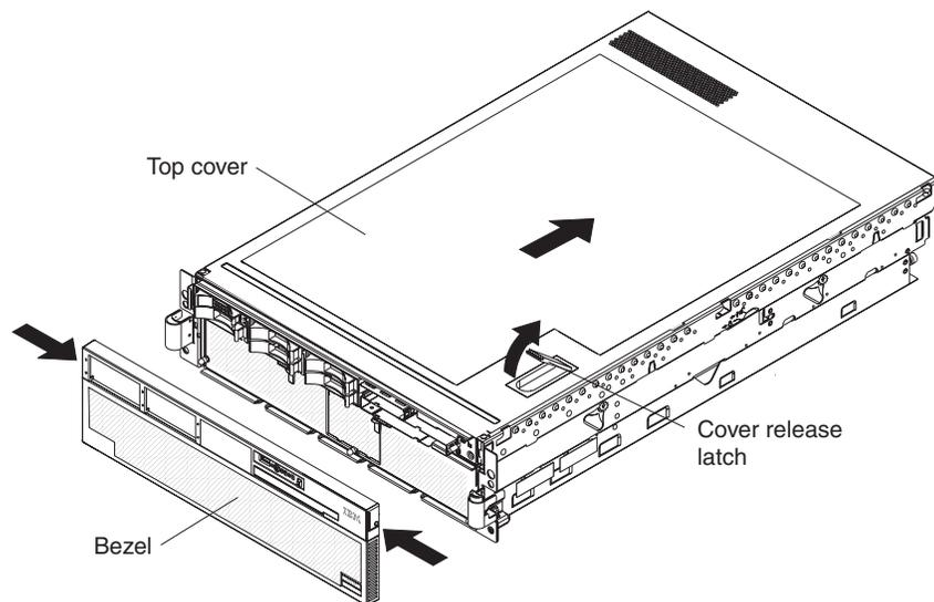
4. Lift the cover-release latch. The cover slides to the rear approximately 13 mm (0.5 inch). Lift the cover off the server.
