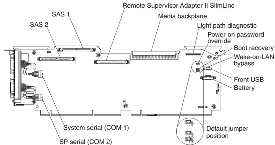
While the server is turned off, move the jumper on J9 from pins 1 and 2 to pins 2 and 3. You can then start the Configuration/Setup Utility program and reset the power-on password. After you reset the password, turn off the server again and move the jumper back to pins 1 and 2.
