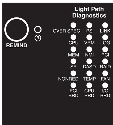
Look at the system service label on the top of the server, which gives an overview of internal components that correspond to the LEDs on the light path
