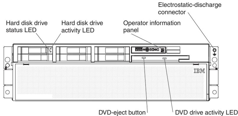
**Hard disk drive status LED:** If a ServeRAID-8i adapter is installed, when this LED is lit it indicates that the associated hard disk drive has failed. If the LED flashes slowly (one flash per second), the drive is being rebuilt. If the LED flashes rapidly (three flashes per second), the controller is identifying the drive.
