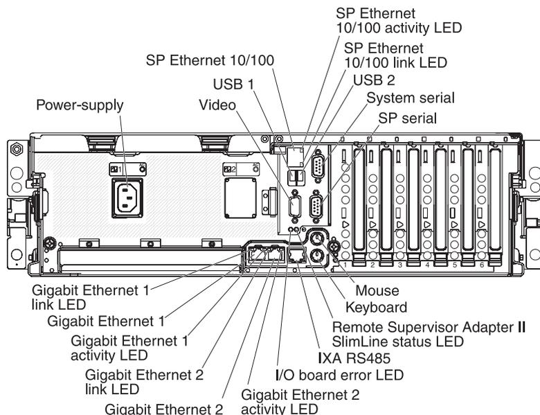
**Power-supply connector:** Connect the power cord to this connector.
