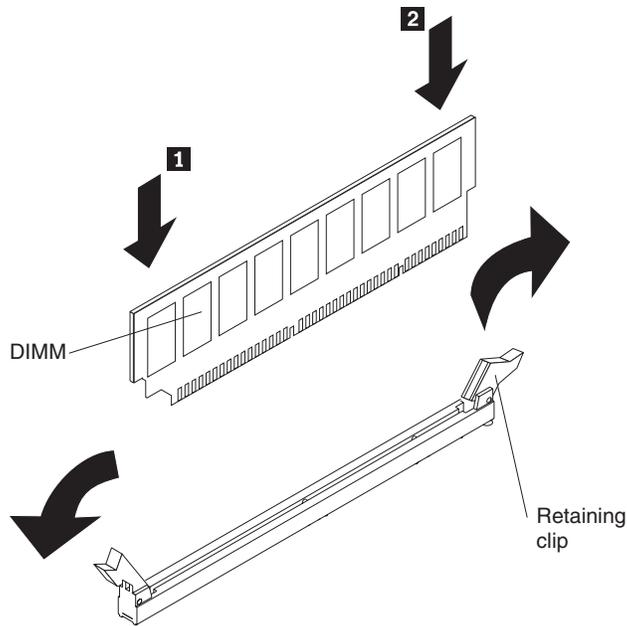
8. Insert the DIMM into the connector by aligning the edges of the DIMM with the slots at the ends of the DIMM connector.
