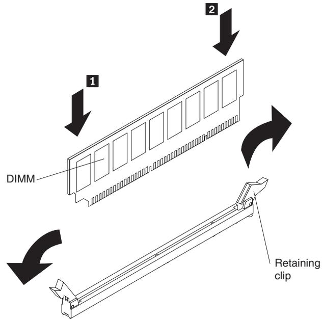
7. Insert the DIMM into the connector by aligning the edges of the DIMM with the slots at the ends of the DIMM connector.
