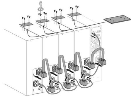
Figure 16. Installing four EBMs (tower)
