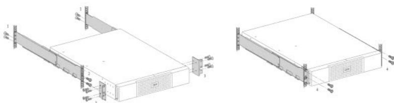
Figure 12. Rack installation using rails
