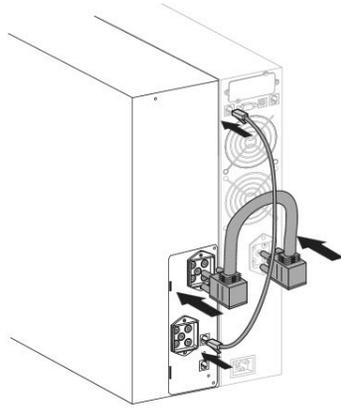
Figure 15. Installing one EBM (tower)
