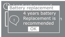
Replace all battery packs in the UPS and any EBMs connected to the UPS at the same time. The replacement battery packs must have no more than 12 month variation between their dates of manufacture and should not have reached or exceeded their shelf life. Dispose of battery packs in accordance with local regulations.
