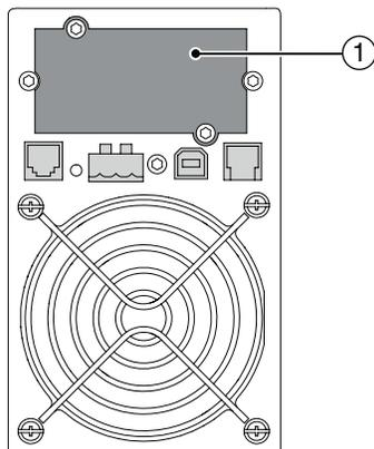
1. Remove the connector panel blank (1), which is secured by two screws.
