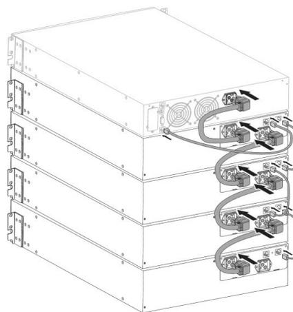
Figure 14. Installing four EBMs (rack)
