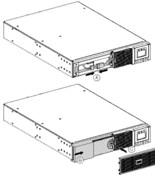
1. Remove the two bezel sections.
