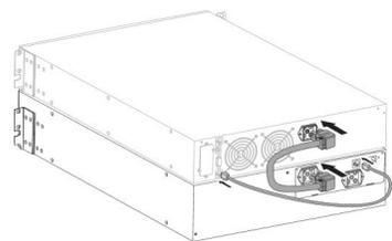
Figure 13. Installing one EBM (rack)
