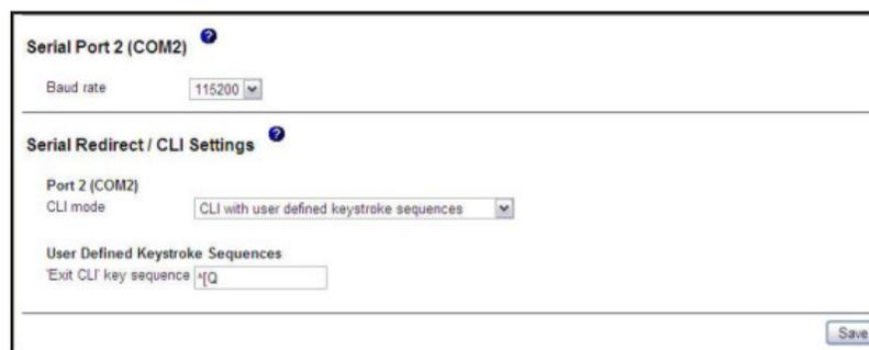
The screenshot displays the configuration page for Serial Port 2 (COM2). It includes a 'Baud rate' dropdown menu currently set to 115200. Below this is the 'Serial Redirect / CLI Settings' section, which contains a 'Port 2 (COM2) CLI mode' dropdown menu set to 'CLI with user defined keystroke sequences'. There is also a 'User Defined Keystroke Sequences' section with a text input field containing 'Exit CLI key sequence |rQ'. A 'Save' button is located at the bottom right of the form.
