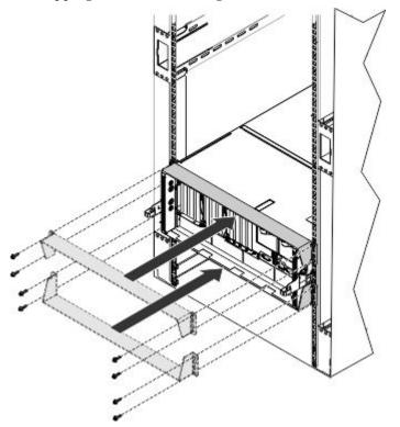
4. Install four M5 combi-head screws (black) from the shipping bracket kit in the bottom shipping bracket, two screws on the right side and two screws on the left side.
