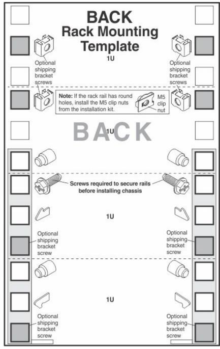
**3**. Install the M5 cage nuts (for square holes) or M5 clip nuts (for round holes) from the shipping bracket kit in the holes that are indicated on the template, if shipping the server in a pre-installed rack.
