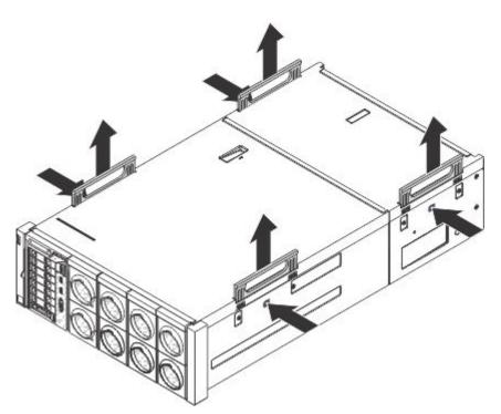
**3. Attention:** To ensure proper installation of the server, do not push the rear lift handles into the rack until the server is securely on the rails in the rack. When removing the server from the rack while sliding the server forward, eject the lift handles as soon as they are clear from any server immediately above the one you are removing.
