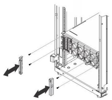
7. Install four M5 combi-head screws (black) through the front of the server (two screws on each side).
