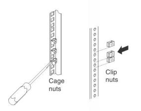
4. Repeat steps 2 on page 5 and 3 on page 7 for the rear of the rack. Make sure that a cage nut or clip nut is installed in every hole indicated on the template.
