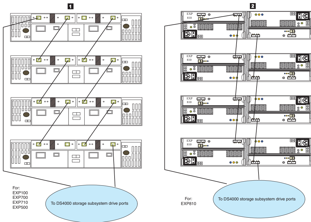
Figure 36. Best practice cable loop scheme for connecting storage devices
