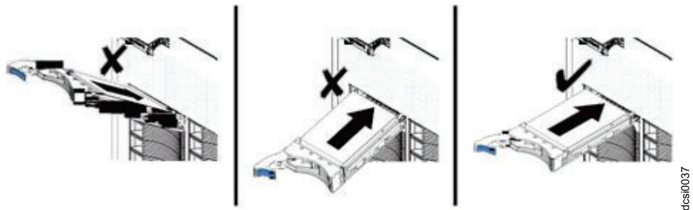
Figure 77. Inserting a hard disk drive into a drive slot
