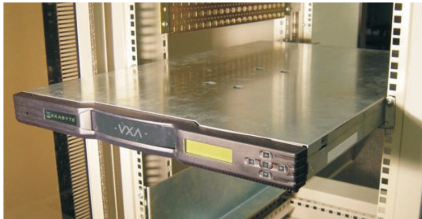
Figure 10. Placing the autoloader on the rails
