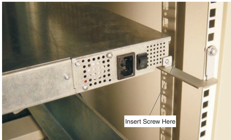
Figure 11. Attaching the autoloader to the rails
