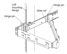
2. Pull back on the blue hinge-pin actuator on the ramp assembly and place the hinge pins of the ramp assembly into the matching hinges of the right-slide rail. Push the hinge-pin actuator forward to securely engage the hinge pins.
