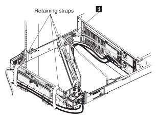
5. Secure the cable-restraint bracket **1** to the slide rail.
