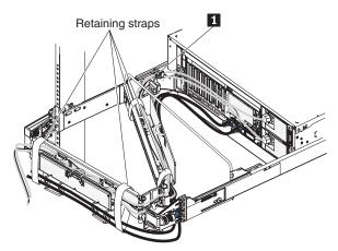
6. Secure the cable-restraint bracket **1** to the slide rail.
