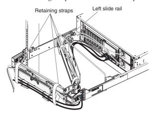
5. Slide the server in and out of the rack to make sure that the ScaleXpander cables remain in the wire-form clips.
