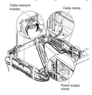
**Note:** When disconnecting the cables from the server, carefully push down on the blue tabs, then pull the cables out of the connectors.
