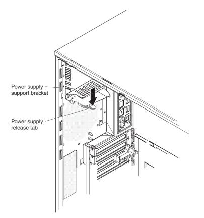
**13**. Raise the power-supply cage slightly and press and hold the release tab on the rear power-supply support bracket; then, lower the power-supply structure into position. For clarity, the power-supply cage is not shown in the illustration.
