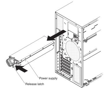
9. Remove the power supply and power-supply filler from the server by pressing down on the release latch while you pull out.
