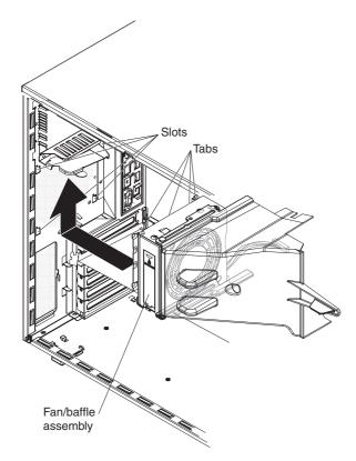
**c**. Carefully flex the air baffle so that you can position it over the pins on the fan cage assembly. Attach the air baffle to the fan cage assembly, then pivot the air baffle and slide it into position on the fan cage assembly.
