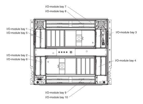
As of the date of this document, Fibre Channel I/O modules, such as the following types of I/O modules, can be installed only in I/O-module bays 3 and 4 of the BladeCenter unit, or in a device, such as the Multi-Switch Interconnect Module, in the high-speed I/O-module bays of the BladeCenter H unit:
