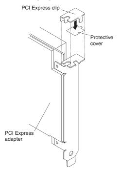
To install a PCI Express adapter clip on a PCI Express adapter, complete the following steps:
