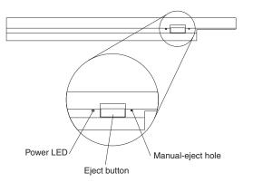
Power LED: This LED is lit when the drive is in use.
