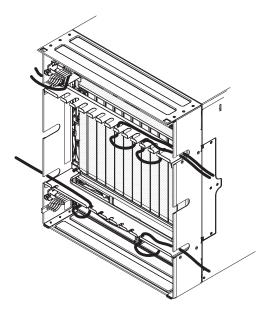
9. Route the cables through the cable management trays and through the slots on either side of the bezel collar.
