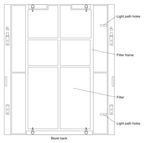
2. Lay the bezel on a flat work surface and orient it so that the bottom of the bezel is closest to you and the light path holes are to the right. The large rectangles in the filter frame should be closest to you.
