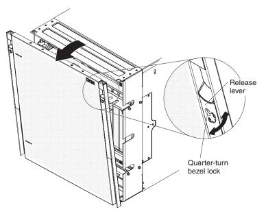
1. Using a small flat-blade screwdriver, unlock and remove the bezel from the BladeCenter HT unit.
