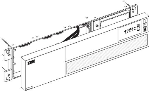
**Important:** Before you move the uninterruptible power supply to another location, make sure that you disconnect the uninterruptible power supply internal battery.
