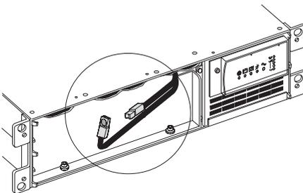
4. Install the uninterruptible power supply front bezel.
