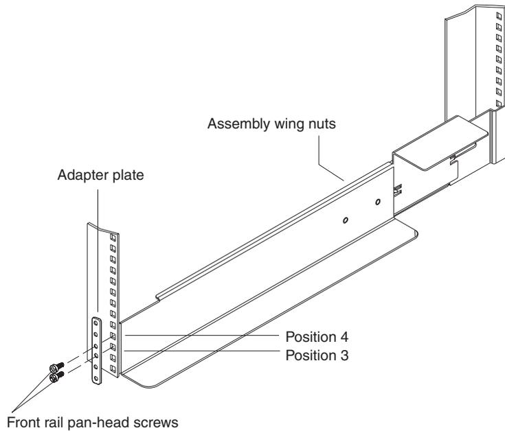
6. Attach the rail to the front of the rack cabinet with two #10-32 pan-head screws.
