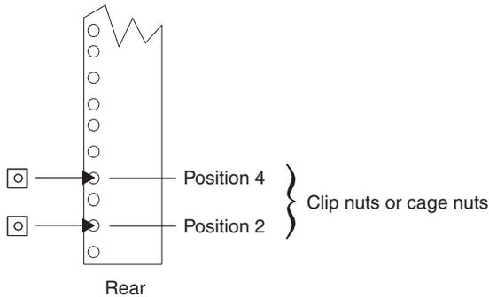
4. Attach the rail to the rear of the rack cabinet using two M5 (hex-head) screws.
