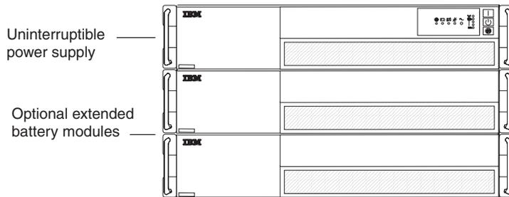
11. Secure the front of the uninterruptible power supply or extended battery module to the rack cabinet using four #10-32 pan-head screws.
