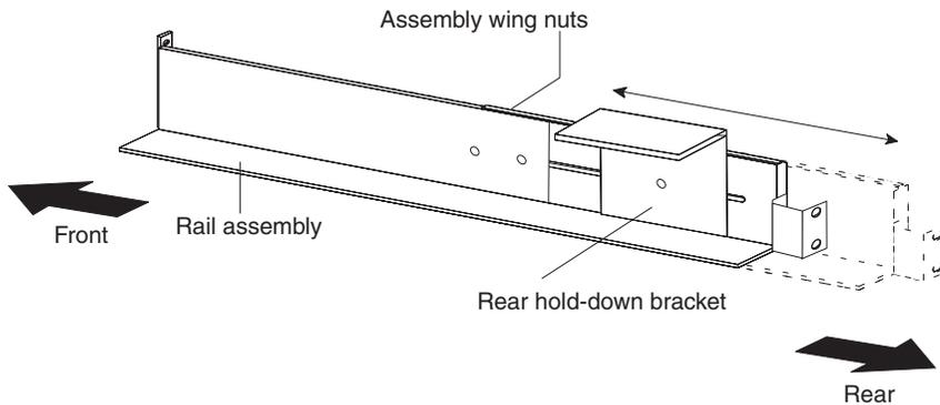
2. If you are shipping the rack cabinet with the uninterruptible power supply and extended battery modules installed, you must secure the units in the rack cabinet with the rear hold-down brackets that come with the rail kit. To attach the rear hold-down bracket to the rail assembly, align the bracket toward the rear of the rail and attach it with one wing nut from the rail kit.
