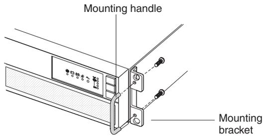
10. Slide the uninterruptible power supply or extended battery module into the rack cabinet. Make sure that you install the extended battery module below the uninterruptible power supply.
