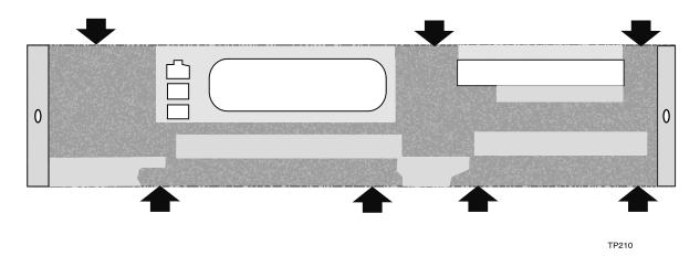
Figure 1. Telco/Industrial Grader Server TIGPR2U Front Filter
