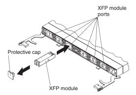
**Attention:** To avoid damage to the cable or the XFP module, make sure that you do not connect the fiber optic cable *before* you install the XFP module.
