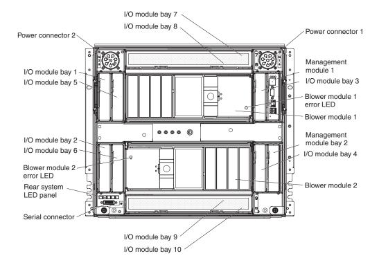
As of the date of this document, the switch module can be installed only in I/O-module bay 7 or 9 of the BladeCenter unit. The other I/O-module bays do not support the switch module.
