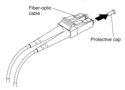
2. Gently slide the fiber optic cable into the XFP module until it clicks into place.
