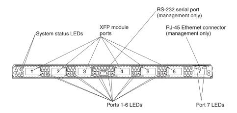
The switch-module information panel contains the following components:
