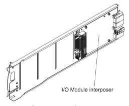
The IBM<sup>®</sup> BladeCenter<sup>®</sup> HT Interposer for Gb Switch/Bridge Bays and IBM BladeCenter HT Interposer for GB Switch/Bridge Bays with Interswitch Links (ISL) option can be installed in I/O bays 1, 2, 3, or 4 for use with Gb switch or bridge modules.
