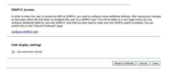
Click **Configure SNMPv3 User** to perform additional user configuration that is required for SNMPv3 (see "Configuring SNMP" on page 23 for instructions). If automatic refresh for **Web display settings** is enabled for a user profile, all advanced management module user interface web pages that have auto-refresh capability will be automatically refreshed during web sessions for the user. If automatic refresh is disabled, there will be no automatic refresh for web sessions of this user.
