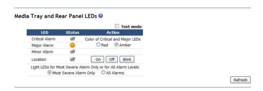
Select **LEDs** to view the state of the BladeCenter T or BladeCenter HT system-status page and blade server control panel LEDs. You also can use this choice to turn on, turn off, or flash the location LED on the BladeCenter unit and the blade servers, and control how the LEDs respond to alarms.
