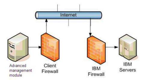
In this setup, the advanced management module connects through the client-provided Internet connection by the default route. For the advanced management module to communicate successfully, your external firewall must allow established TCP packets to flow freely on port 443 (HTTPS).
