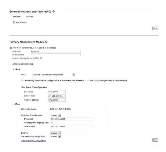
**Attention:** Once IPv6 has been enabled, disabling it or updating advanced management module firmware to a level that does not support IPv6 addressing causes all IPv6 connectivity to be lost. Services and interfaces that are configured for IPv6 operation might not function properly and you will need to reconfigure these services and interfaces.
