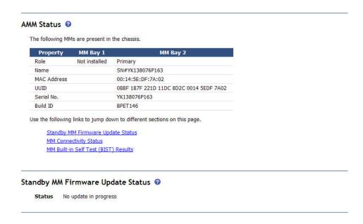
The **Standby MM Firmware Update Status** section displays the status of the firmware update, versions of the firmware images, percent complete, and estimated time to complete the update of the standby management-module firmware.
