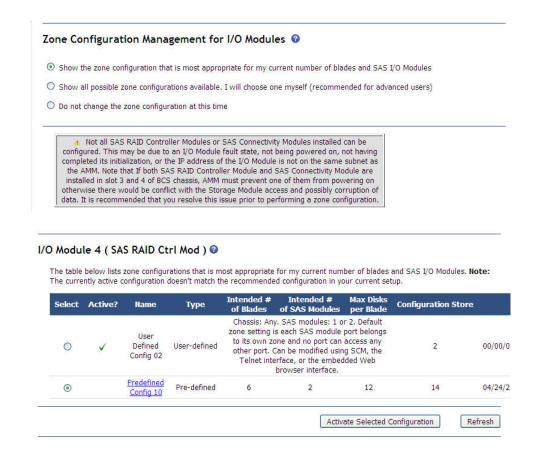
When both RAID and non-RAID storage modules are installed, only one module can be powered-on at a time and have its zone configuration managed. If multiple SAS modules are installed and both are working, make sure that the default setting
