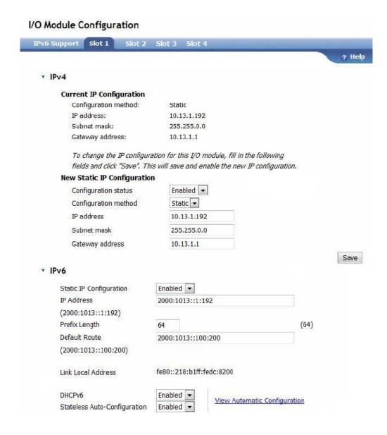
When you use the management-module web interface to update an I/O-module configuration, the management-module firmware writes its settings for the I/O module only to the management-module NVRAM; it does not write its settings for the I/O module to the I/O-module NVRAM.
