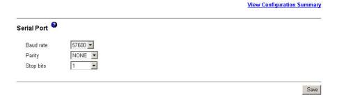
You can configure the serial port settings for baud rate, error checking parity, and the number of stop bits. Connections that are made using the advanced management-module serial port can access only the management-module CLI and the Serial over LAN (SOL) feature. See the *BladeCenter Advanced Management Module Command-Line Interface Reference Guide* for information about using the serial port.
