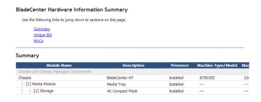
Select Monitors > Hardware VPD to view the VPD for the BladeCenter unit. When the BladeCenter unit is started, the management module collects the vital product data and stores it in nonvolatile memory. The management module then modifies
