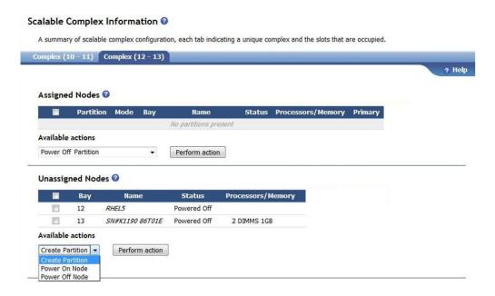
The following **Available actions** can be applied to a selected blade server node by clicking **Perform action**. Select one or more nodes in a complex using its check box.
