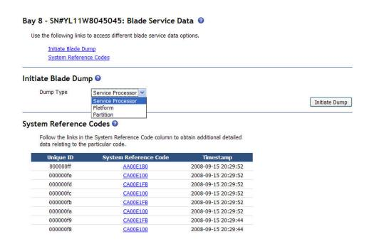
To show the details of a system reference code, click the system reference code link. A page that contains the details of the selected system reference code is displayed.
