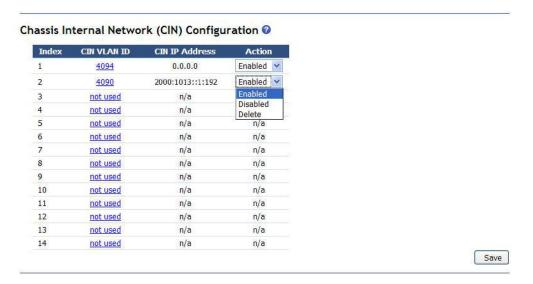
Each CIN interface to the advanced management module has an associated index number, ID, IP address, and action value.
