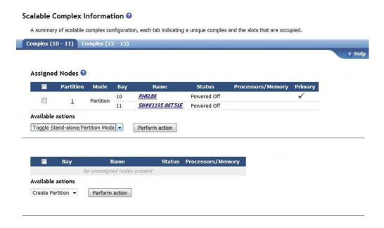
In a scalable complex, each node is a blade server. The blade server nodes can be grouped into partitions that function as a single system and share resources. The name of each node is a link to detailed information about the blade server it represents.
