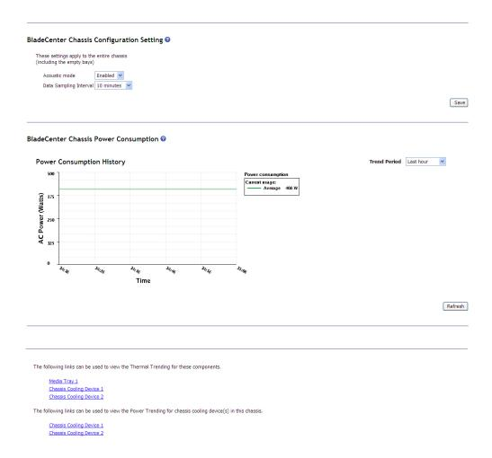
The **BladeCenter Chassis Configuration Setting** section configures how the management module responds if it detects an over-temperature condition (thermal event) on a blade server. The following acoustic mode options are supported in response to thermal events:
