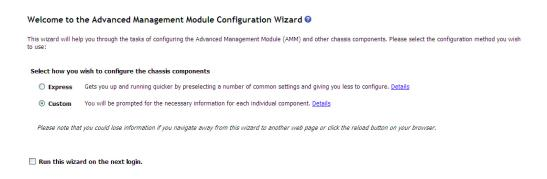
The configuration wizard repackages the information in the other advanced management module pages into a structured flow that facilitates the configuration process. See "Using the configuration wizard" on page 19 for information about using the configuration wizard.
