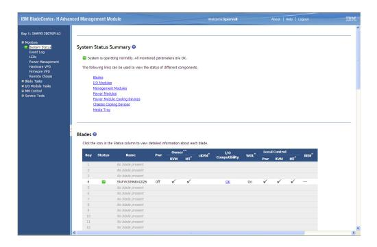
The top of the management-module web-interface page shows the type of management module that you are logged in to. The following illustrations show the management-module types for a management module and advanced management module. Information about configuring management modules other than the advanced management module is in a separate document.
