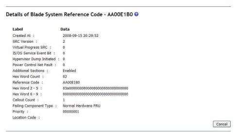
The information on this page can be used by support personnel to diagnose issues. See the *Problem Determination and Service Guide* for assistance with interpreting the codes and detailed data.
