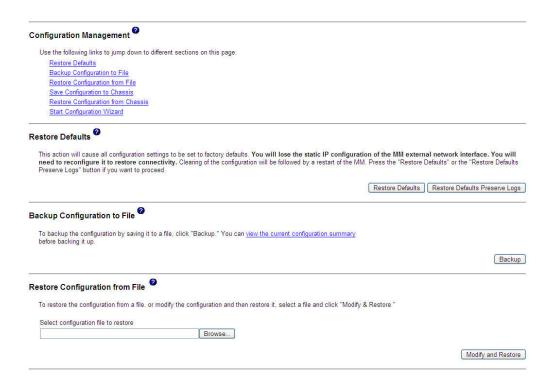
The advanced management module provides several backup and restoration options, including use of a compressed configuration file for BladeCenter units other than BladeCenter H units. (BladeCenter H units compress backups automatically.) When you restore defaults, you can choose to save or discard the management-module event log. See "Using the configuration file" on page 65 for instructions.
