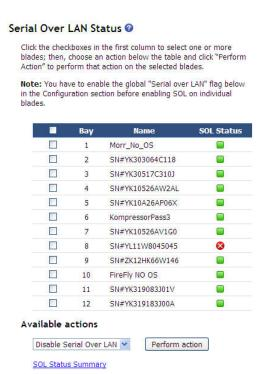
Select **Serial Over LAN** for each blade server and globally for the BladeCenter unit. Enabling or disabling SOL globally does not affect the SOL session status of each blade server; SOL must be enabled both globally for the BladeCenter unit and individually of each blade server on which you plan to start an SOL session. SOL is enabled globally and on the blade servers by default.
