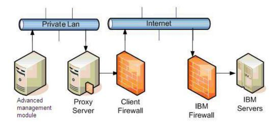
To forward SSL sockets, the proxy server must support the basic proxy header functions (as described in RFC 2616, Hypertext Transfer Protocol 1.1; see http://www.ietf.org/rfc/rfc2616.txt) and the connect method. Basic proxy authentication (RFC 2617, HTTP Authentication: Basic and Digest Access Authentication; see http://www.ietf.org/rfc/rfc2617.txt) can be configured so that the advanced management module authenticates before attempting to forward sockets through the proxy server.
