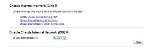
The Chassis Internal Network (CIN) provides internal connectivity between blade server ports and the internal advanced management module management port so that you can access the management module from a blade server by opening a WEB, CLI or SNMP session.
