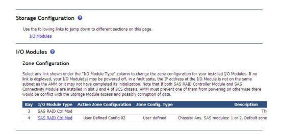
To change the zone configuration for an installed I/O module, click on its link. This will take you to the page you can use to manage the configuration for I/O modules and the optional SAS RAID feature.
