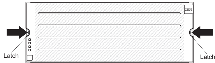
Figure 84. Removing the bezel
