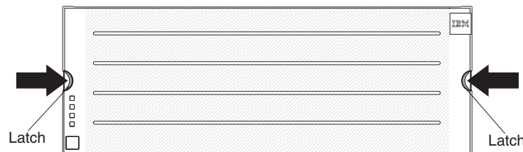
Figure 51. Removing the bezel
