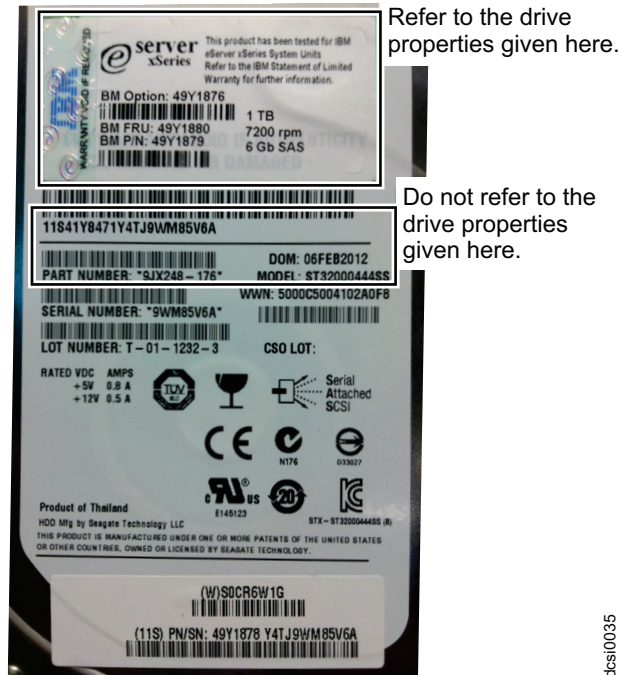
Figure 89. An IBM hologram label example
