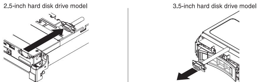
Figure 165. Front video connector removal
