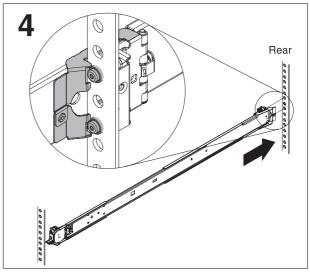
Attach the rear rackmount bracket to the rear of the rack.
