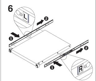
Attach the front rackmount bracket to the front of Attach the inner slide rails to the server. the rack.
