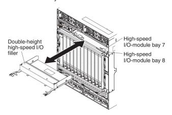
3. Remove the upper and lower interposer filler trays from the BladeCenter unit.
