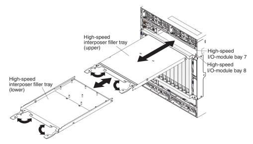
4. Install the upper and lower trays with interposers into the BladeCenter unit.
