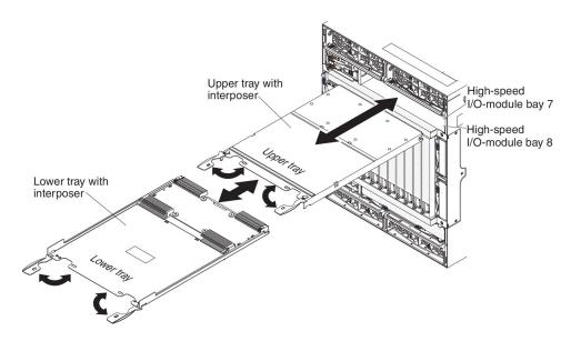
5. Open the orange release handles on the interconnect module by pulling them away from the module.
