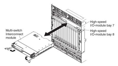
6. Install the interconnect module into the open BladeCenter I/O-bays. Close the release handles to lock the module firmly in place.
