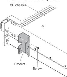
Mount the chassis to rack with two M6 screws which are included in the Enterprise rack rail kit.
