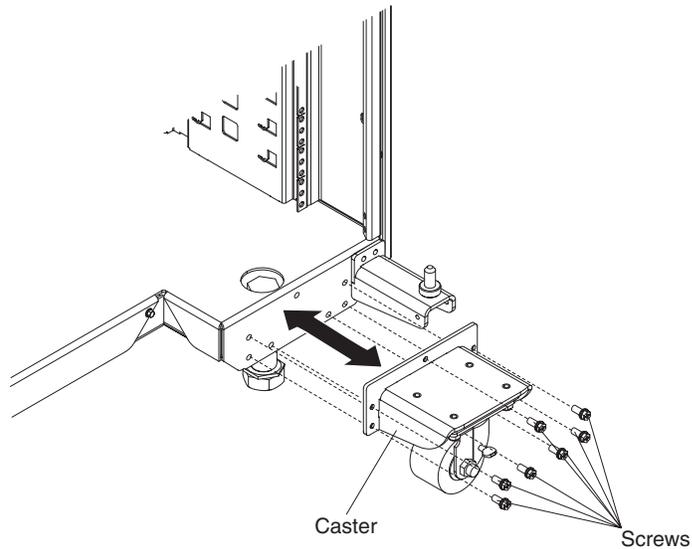
Figure 43. Install and remove the casters
