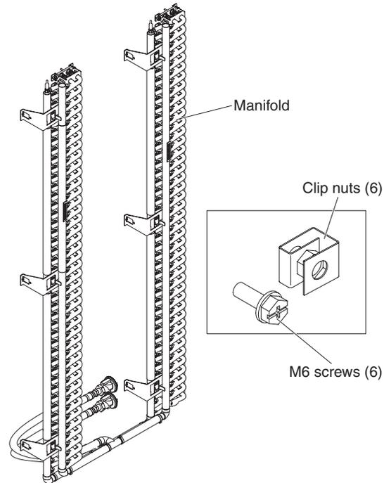
Figure 11. Manifold components
