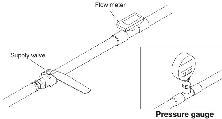
Figure 27. Check the water level with the flow meter
