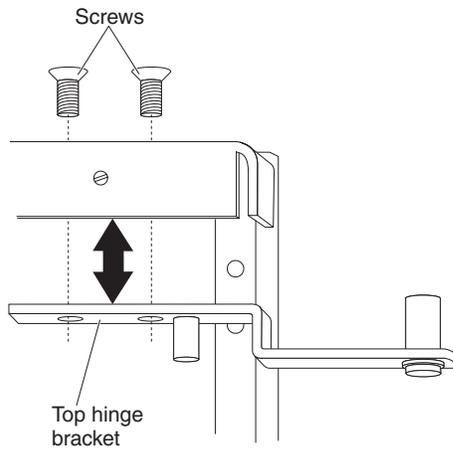
*Figure 24. Install the top hinge bracket*
