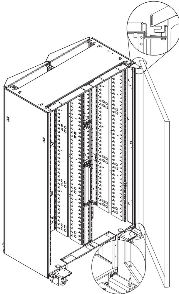
Figure 19. Removing a rear door from the rack cabinet
