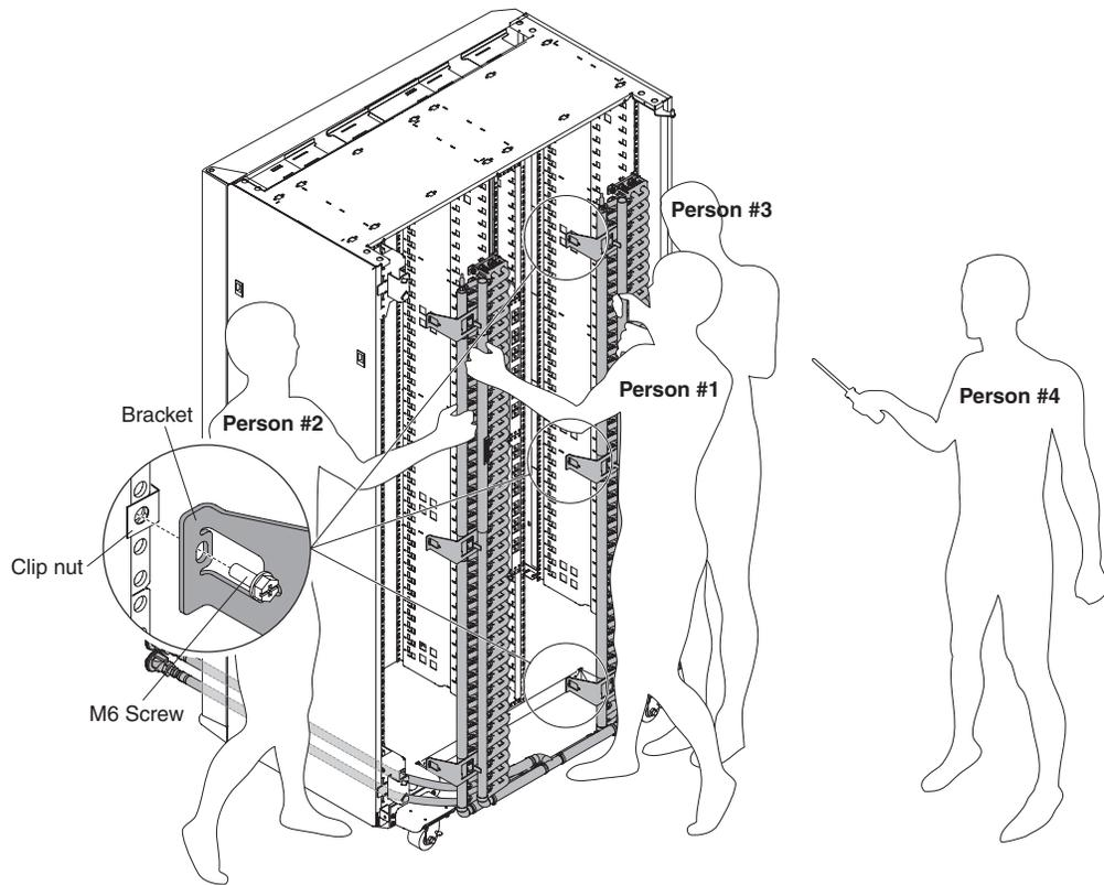
Figure 14. Installing the manifold
