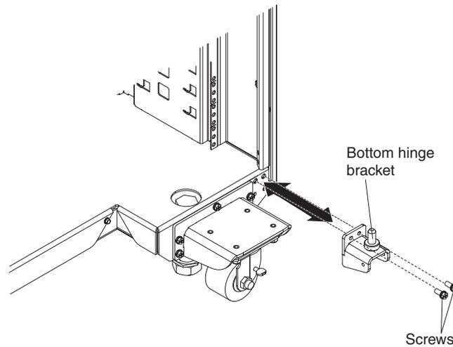
Figure 23. Install the bottom hinge bracket
