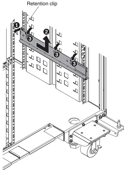
Figure 45. Removing the 2U chassis rails
