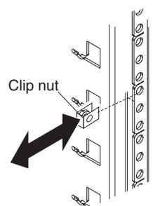
Figure 49. Installing the rear clip nut
