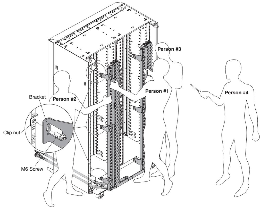
Figure 13. Installing the manifold
