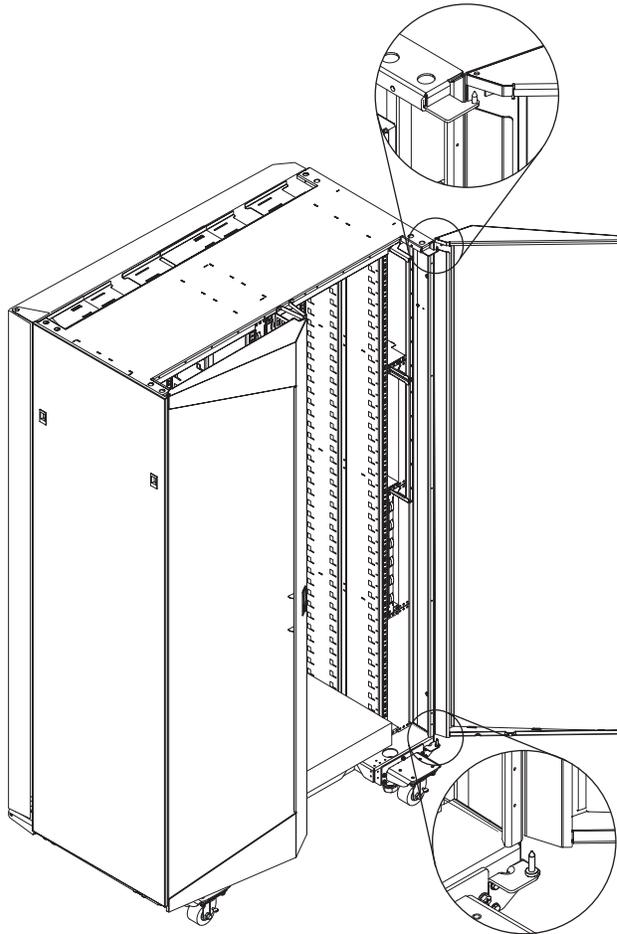
Figure 18. Removing a front door from the rack cabinet
