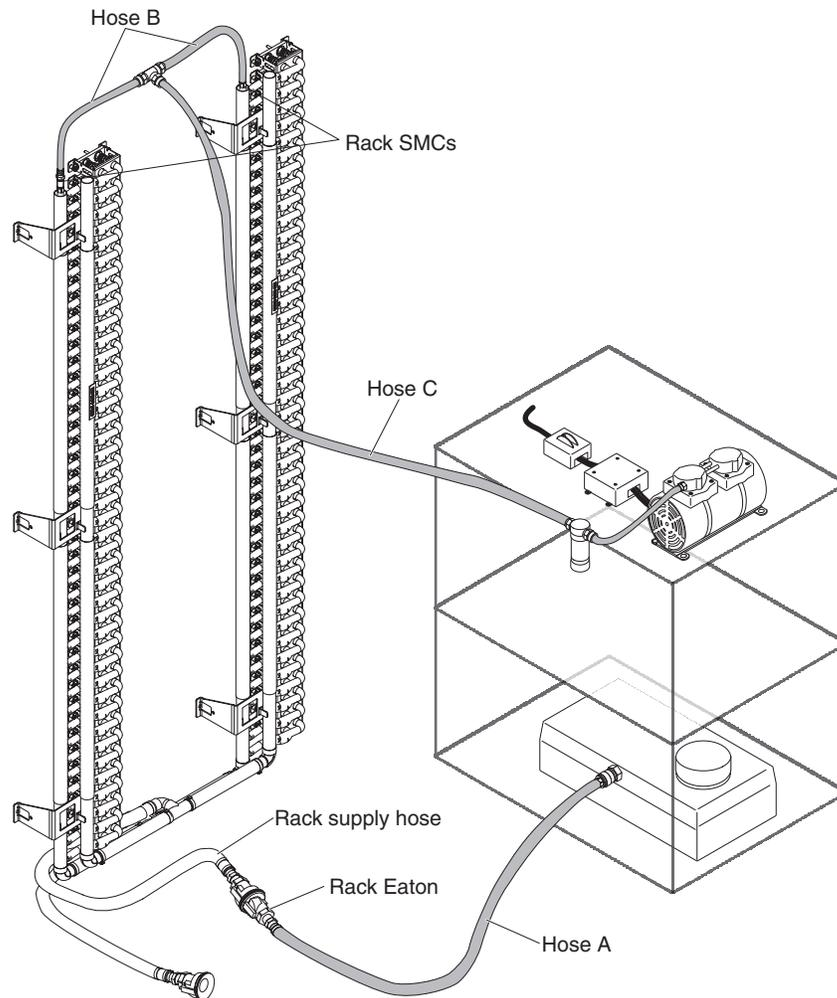
7. All tool hoses can be disconnected from the rack.
