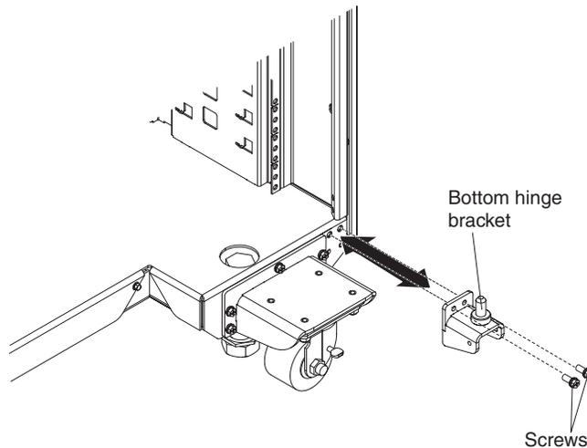
Figure 21. Remove the bottom hinge bracket
