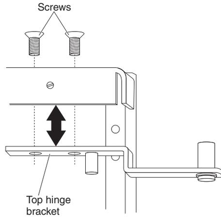
Figure 22. Install the top hinge bracket
