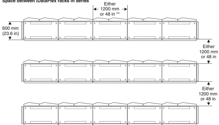
When you attach iDataPlex rack cabinets together to form a suite of rack cabinets, you must keep a minimum distance between suites in the same room. This distance provides proper ventilation and allows access to install and service optional devices.
