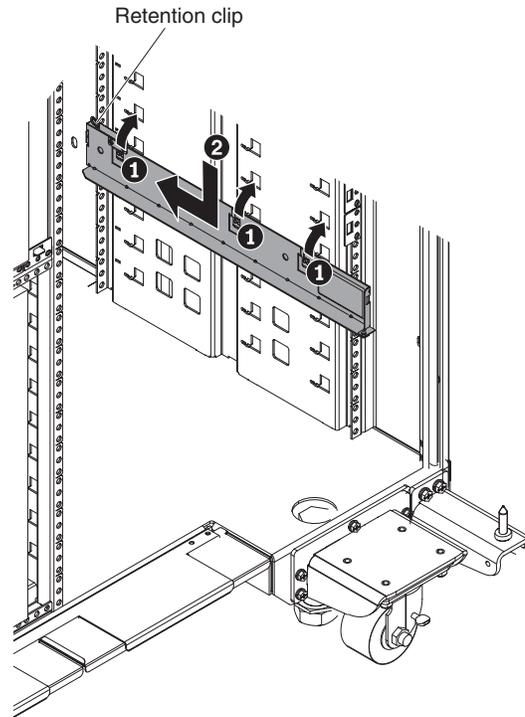
Figure 46. Installing the 2U chassis rail
