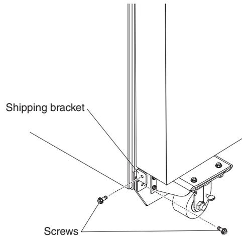
*Figure 8. Removing the rear door shipping bracket*
