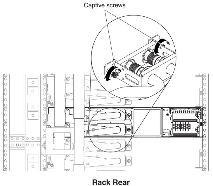
Figure 31. Loosen screws
