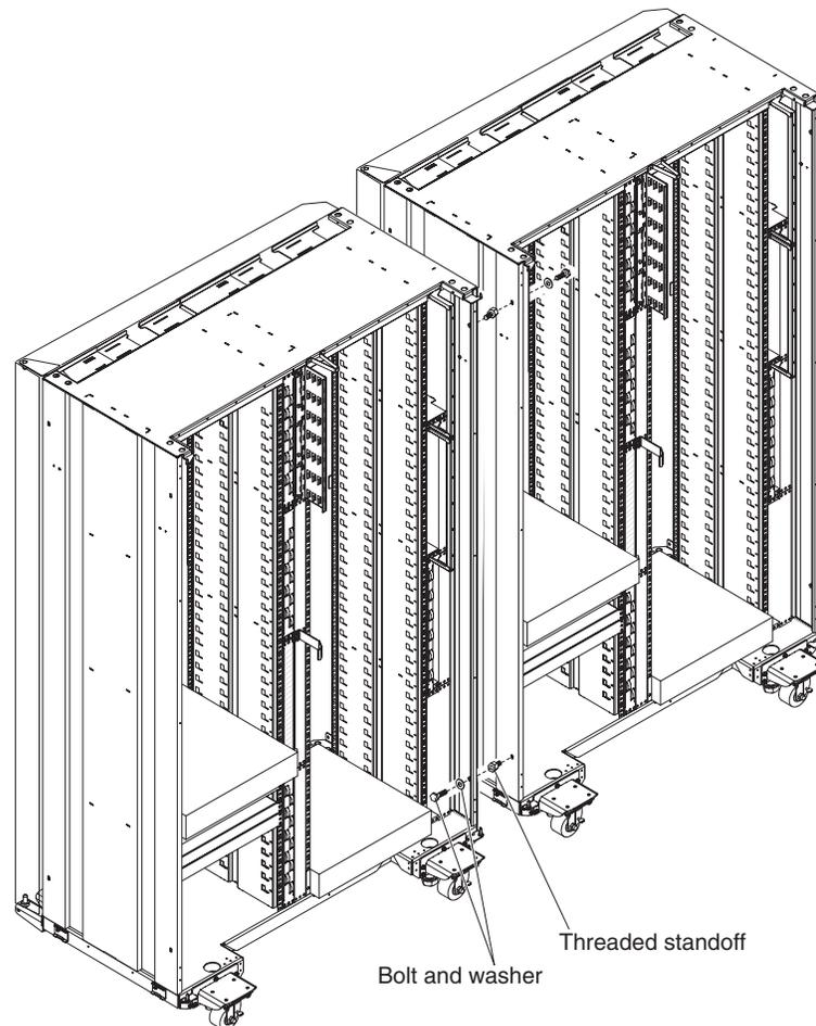
Figure 42. Attaching two adjacent rack cabinets to each other to form a suite
