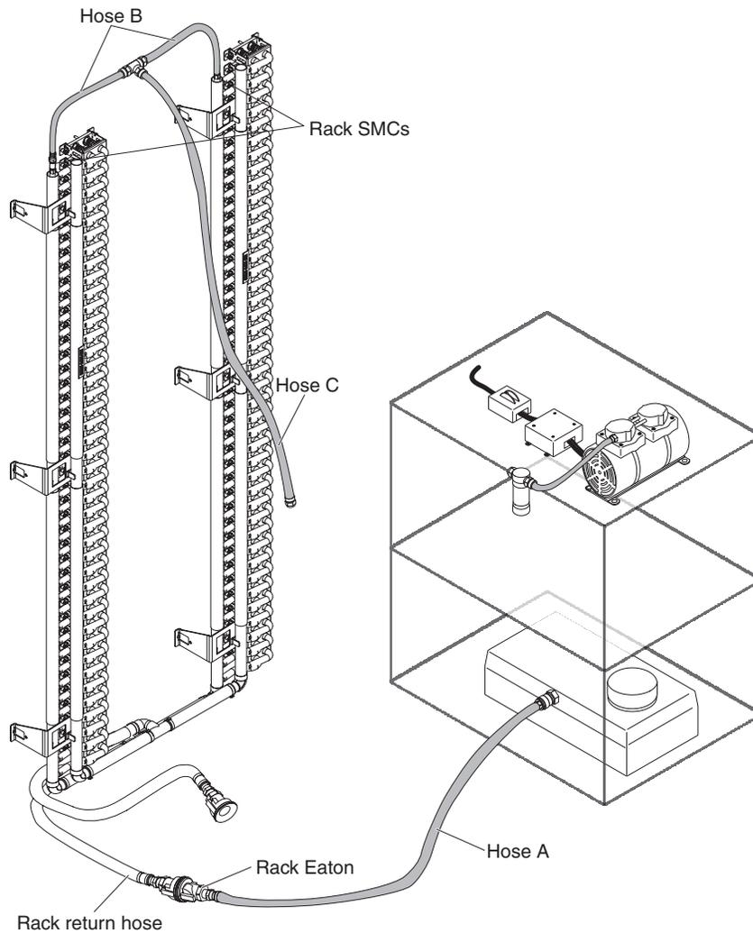
Figure 29. Draining water out of the manifold
