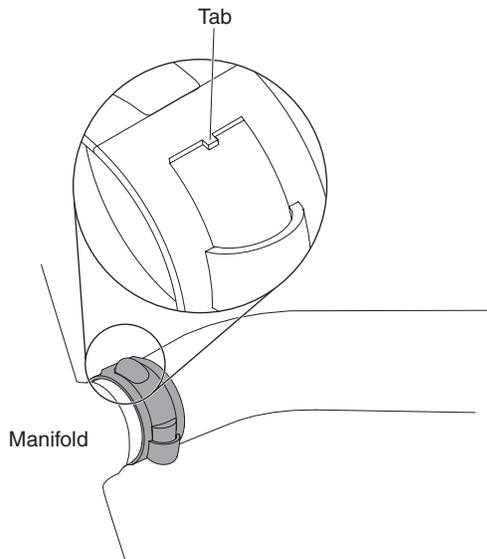
Figure 38. Inspect the clamp
