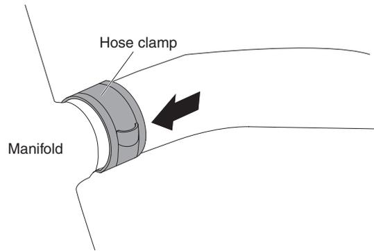
Figure 36. Slide clamp to near the end of the hose
