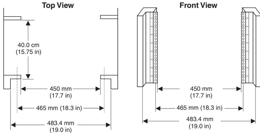
Figure 3. Measuring inside of the rack cabinet
