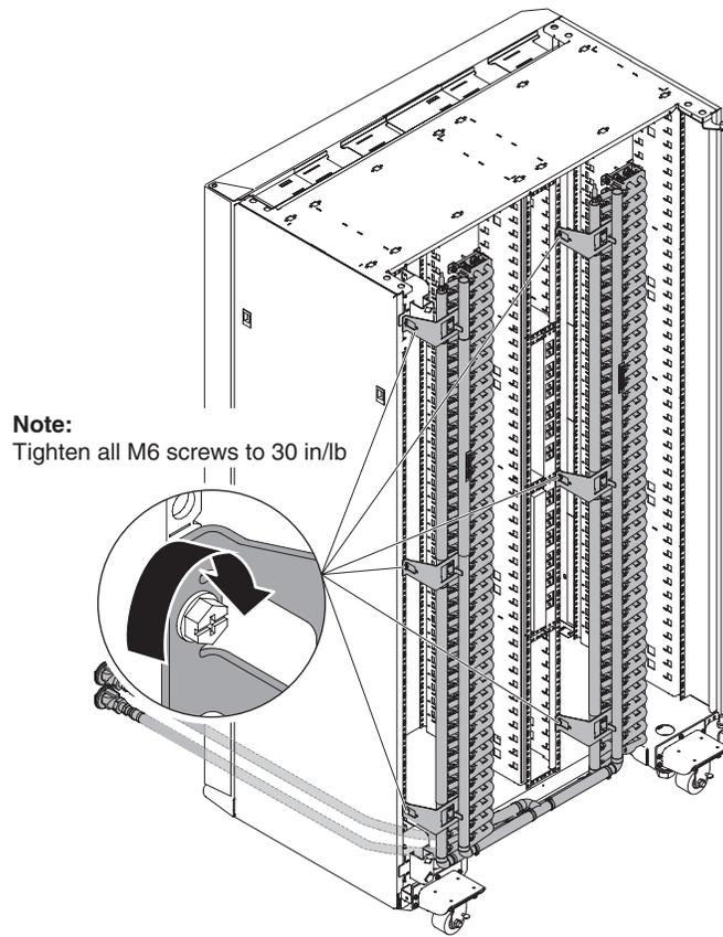
Figure 15. Installing the manifold
