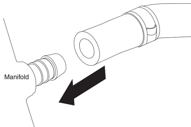
Figure 35. Slide a new clamp into a hose
