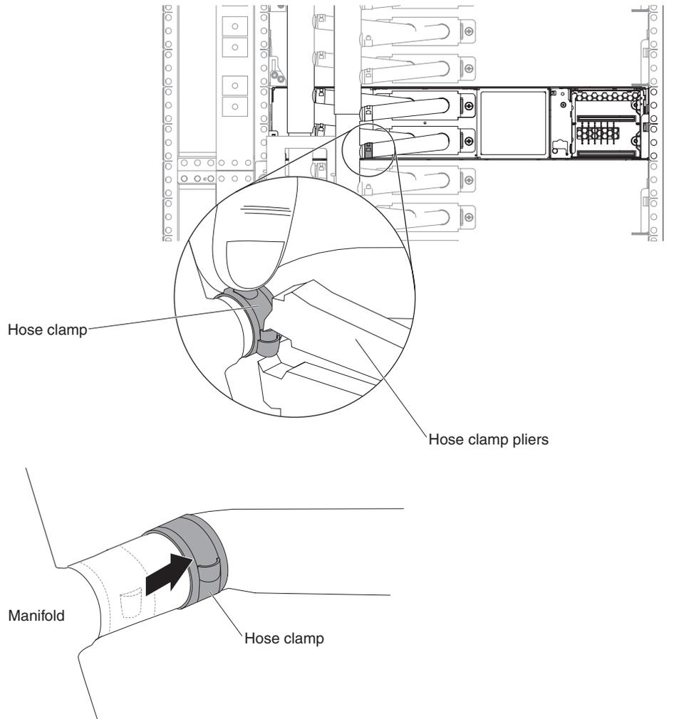
Figure 32. Release the tab at the end of the clamp
