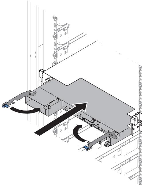
Figure 40. Latch the node back
