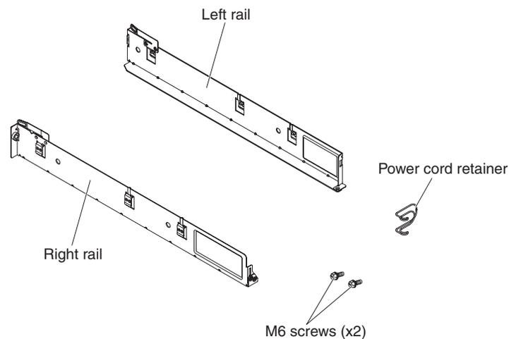
Figure 44. 2U chassis rails
