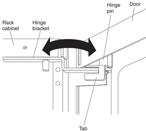
Figure 20. Open the door so that the tab clears the hinge bracket
