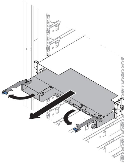
Figure 30. Unlatch the node
