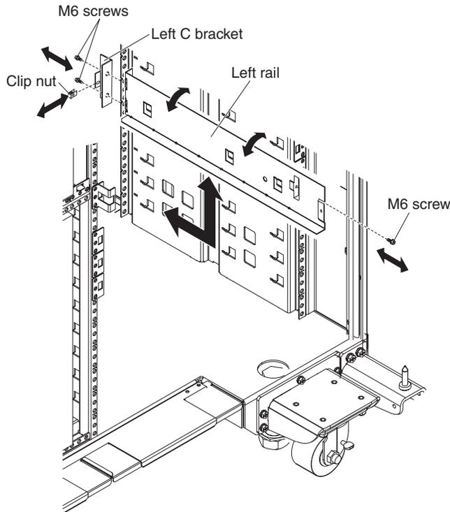
Figure 50. Installing the optional device rails
