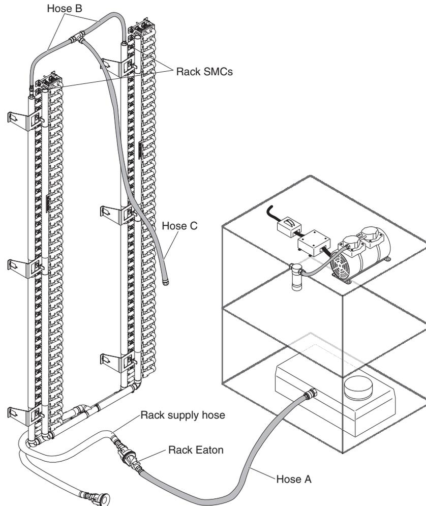
Figure 28. Draining water out of the manifold
