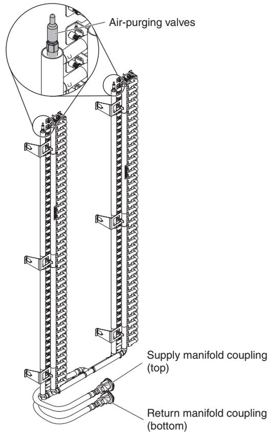
Figure 16. Locations of air-purging valves and drain valve
