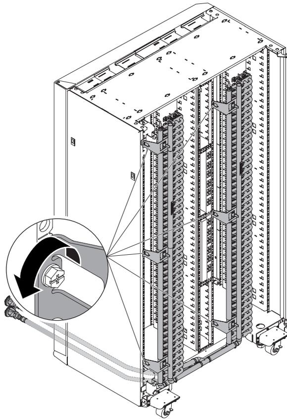
Figure 17. Removing the manifold
