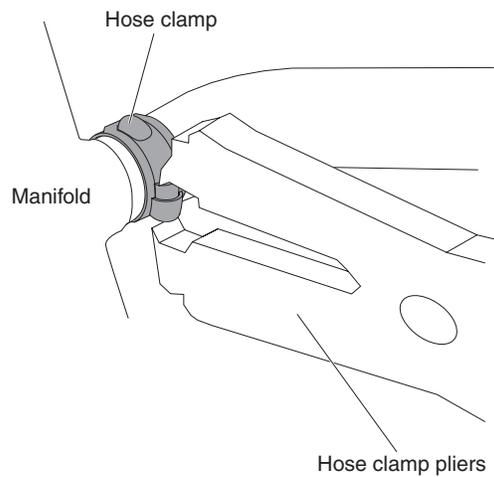
Figure 37. Pinch/squeeze the 2 embosses of the hose clamp
