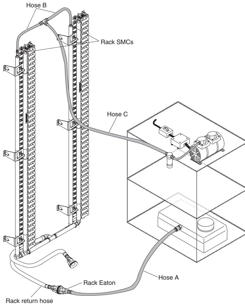
6. With the pump off, disconnect the rack return hose from hose A and replace with the rack supply. Turn the pump on for 3 minutes, then turn off. The manifold should now be adequately drained to allow for any manifold rework.
