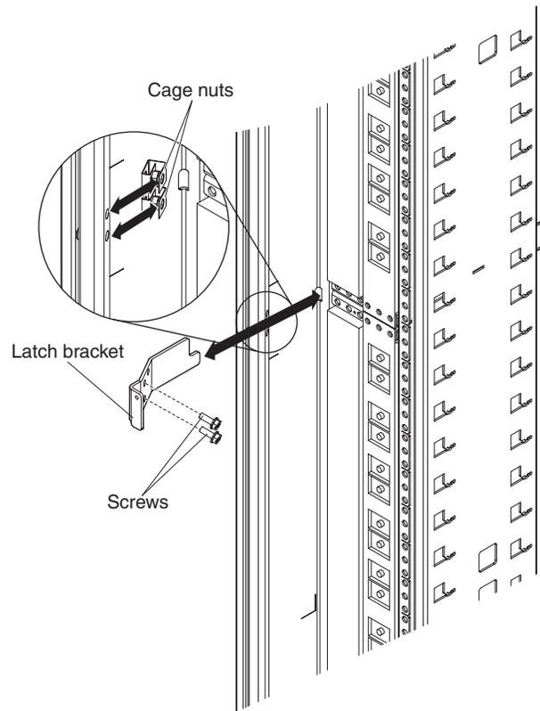
Figure 25. Install the latch bracket
