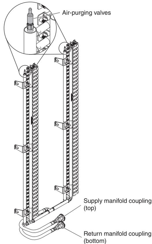
Figure 26. Locations of air-purging valves and drain valve
