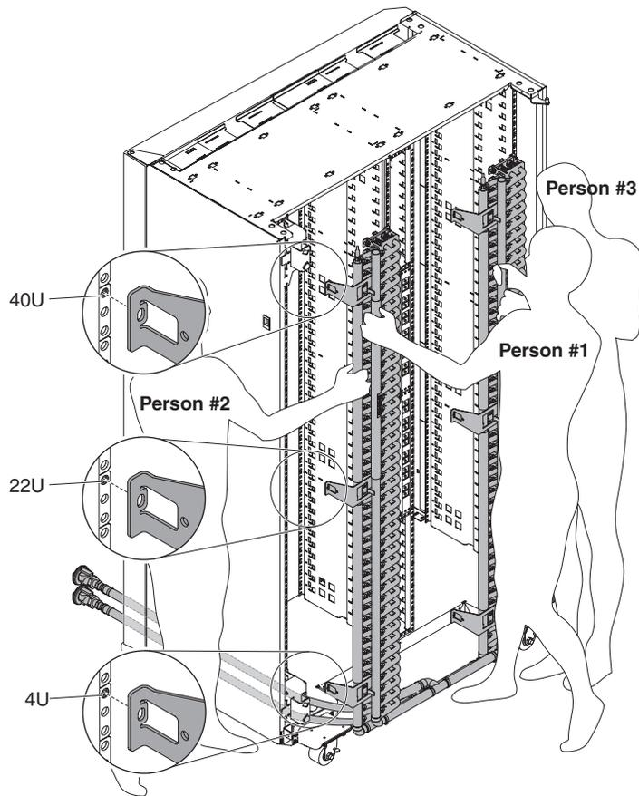
Figure 12. Installing the manifold
