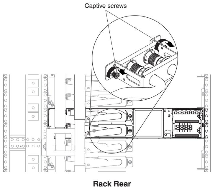
Figure 39. Assemble the hose
