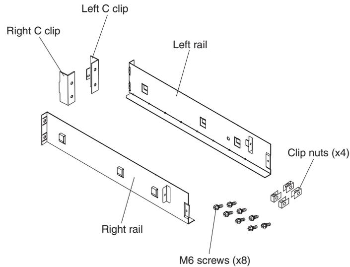
Figure 47. Optional-device rails
