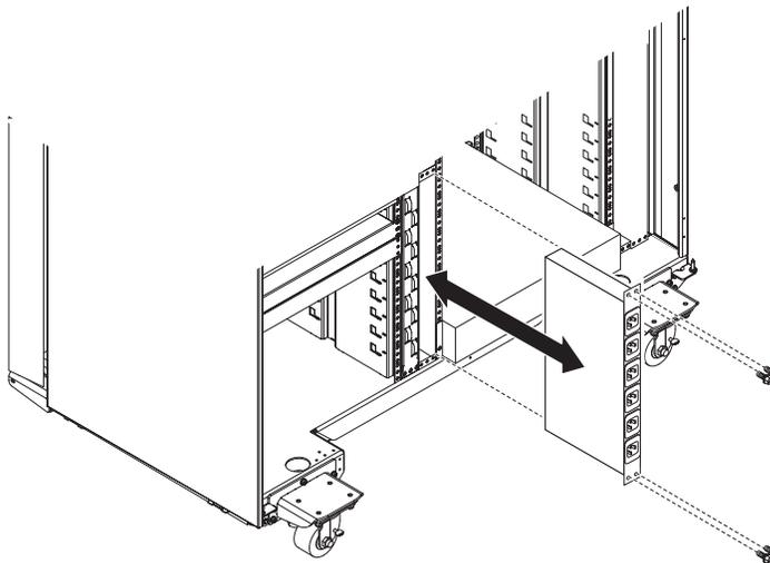
Figure 41. Installing a PDU vertically in a rack cabinet
