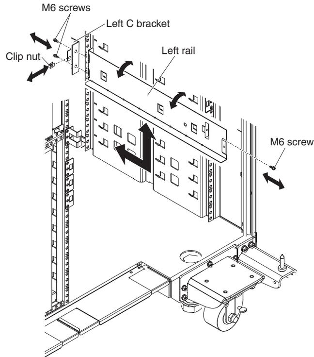
Figure 48. Removing the optional device rails
