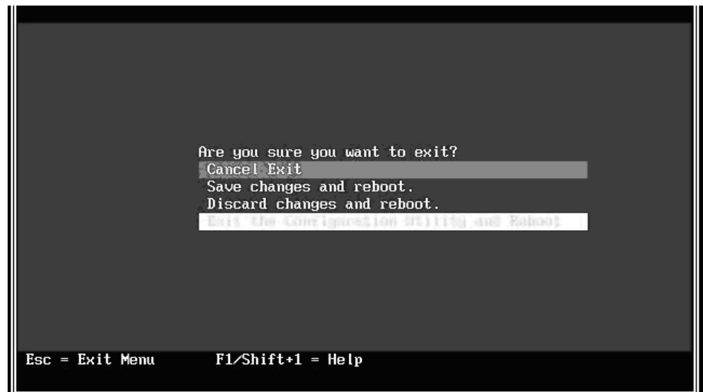
Figure 8. Saving the BIOS setting and rebooting
