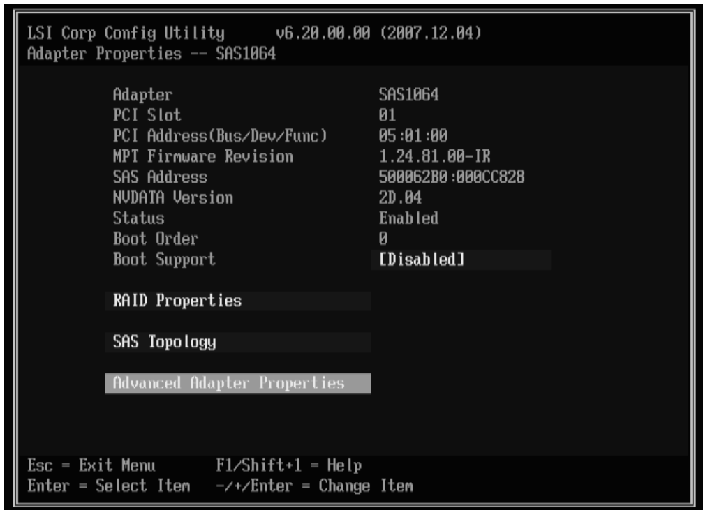
Figure 5. Disabling boot support for the SAS Expansion Card
