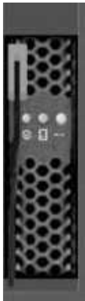
Figure 23. Battery Backup Unit light path indicators
