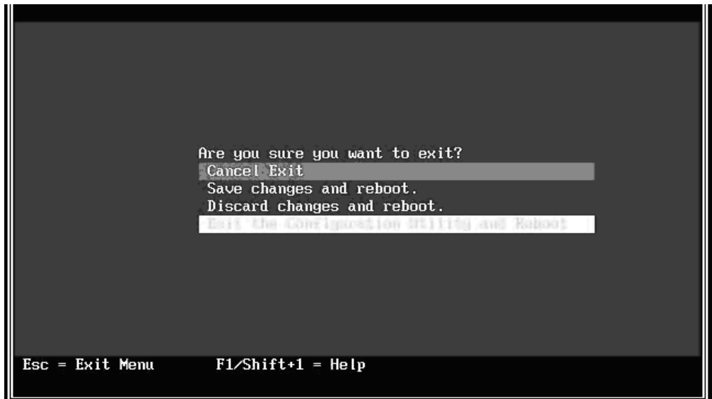
Figure 15. Saving the BIOS setting and rebooting
