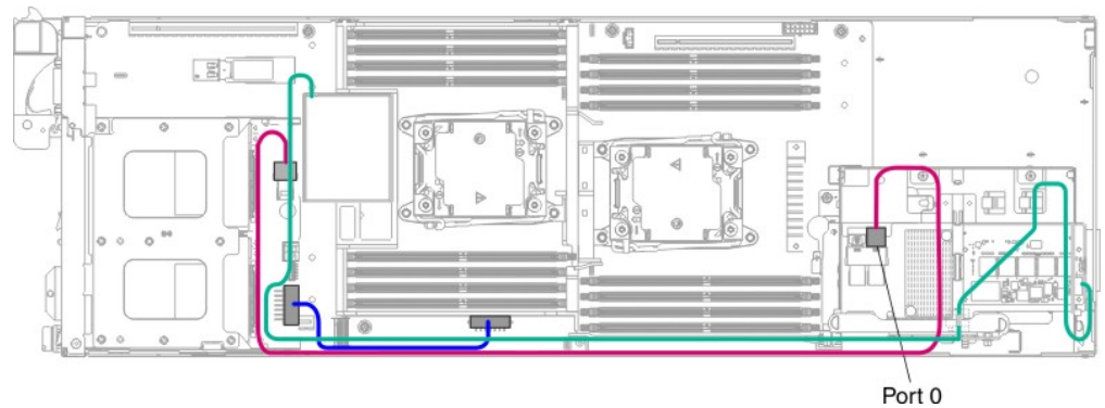
Figure 162. 2.5-inch hot-swap hard disk drive with ServeRAID SAS controller cable connection (no other hard disk drive installed)
