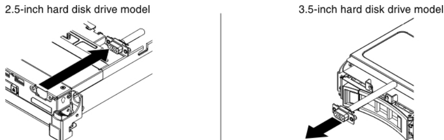
Figure 165. Front video connector removal
