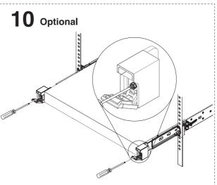
Install the screw in the EIA brackets if needed.
