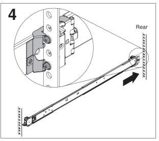
Attach the rear rackmount bracket to the rear of the rack.
