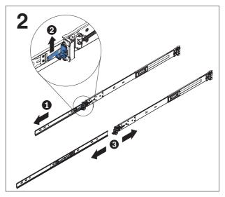
Disassemble the slide-rail assembly.
