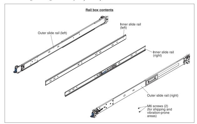
The following illustration shows the items that you need to install the server in a rack cabinet. If any items are missing or damaged, contact your place of purchase.
