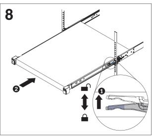
Install the server on the slide rails.
