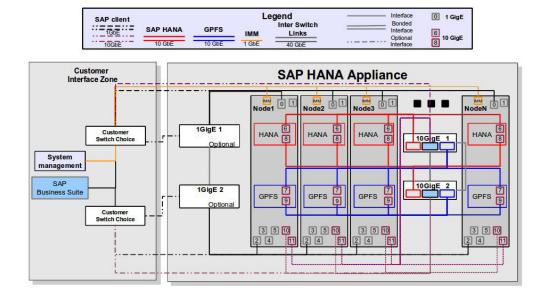
**Note:** The "Customer Switch Choice" labeled switches are either 1 Gigabit Ethernet adapter or 10GbE SFP+ switches provided by you or Lenovo. Make the switch uplink redundant when possible.
