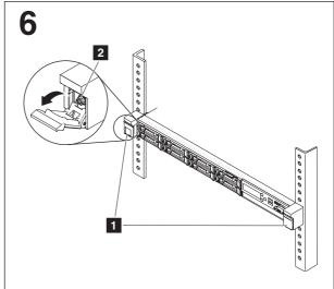
Tighten the front screws if needed.
