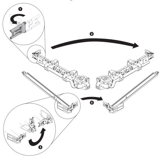
To allow the cable management arm to be installed on the right side of the rack (as viewed from the rear), the stop bracket on the end of the support bar must be rotated to allow the part to be installed on the right slide.
