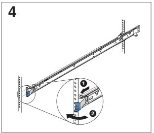
Attach the front rackmount bracket to the front of the rack.
