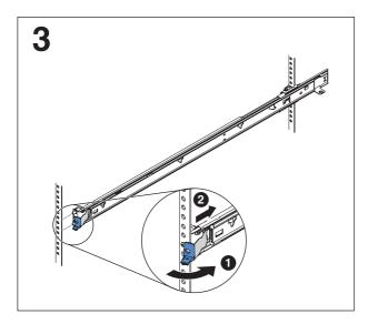
Unlatch the front rackmount bracket from the front of the rack.
