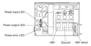
Figure 13. DC power-supply LEDs
