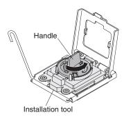
Figure 82. Installation tool handle adjustment
