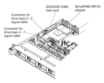
Figure 20. ServeRAID adapter cable connection
