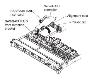
Figure 45. ServeRAID controller installation
