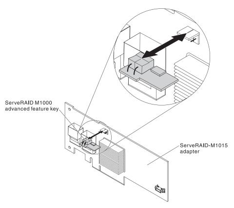
Figure 50. ServeRAID M1000 advanced feature key installation
