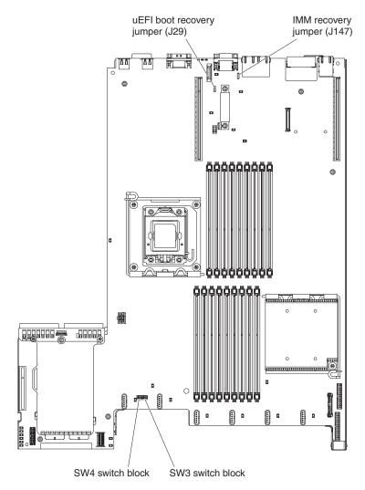
Figure 92. System-board switches and jumpers
