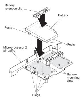
Figure 70. Battery installation
