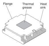
Figure 83. Thermal grease
