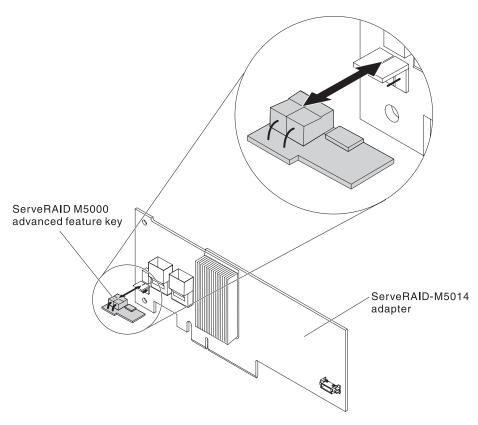
Figure 51. ServeRAID M5000 advanced feature key installation
