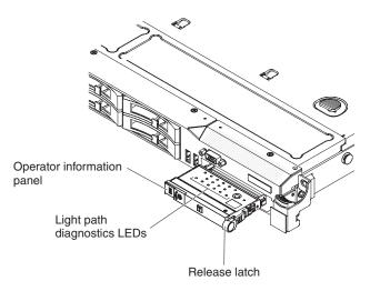
Figure 7. Light path diagnostics panel exposure
