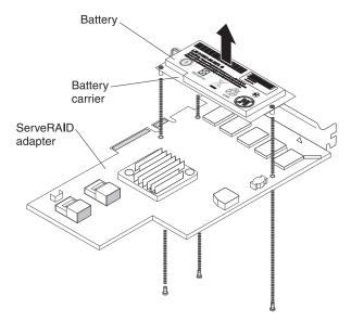
Figure 64. Battery removal
