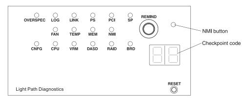
Figure 8. Light path diagnostics panel exposure
