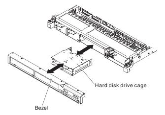
Figure 76. Hard disk drive cage installation
