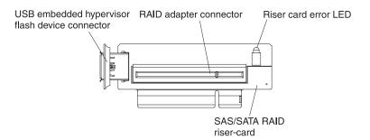
Figure 43. RAID adapter connector
