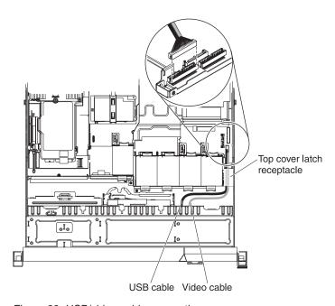
Figure 23. USB/video cable connection
