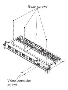
Figure 71. Screws removal
