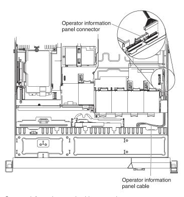
Figure 22. Operator information panel cable connection
