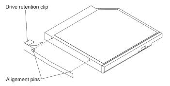
Figure 38. DVD drive retention clip installation
