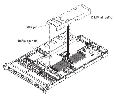
Figure 27. DIMM air baffle removal
