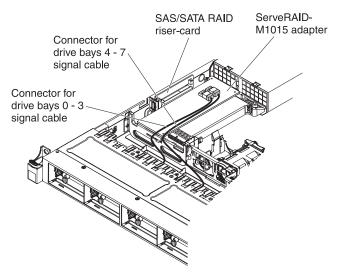
Figure 48. ServeRAID-M5015 adapter cable connection
