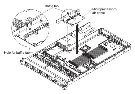
Figure 87. Microprocessor 2 air baffle installation
