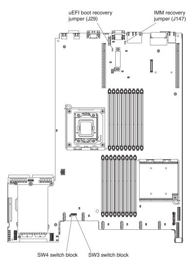
Figure 17. System-board switches and jumpers
