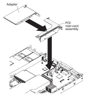
Figure 42. Adapter installation
