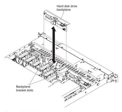
Figure 77. Hard disk drive backplane installation
