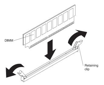
Figure 32. DIMM installation
