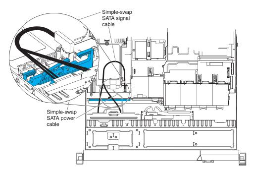
Figure 24. Simple-swap backplate assembly cable connection
