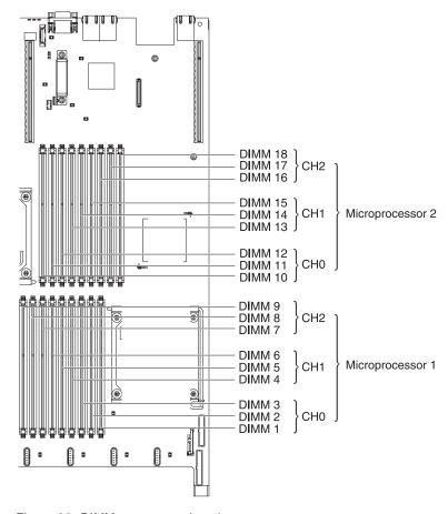
Figure 29. DIMM connectors location
