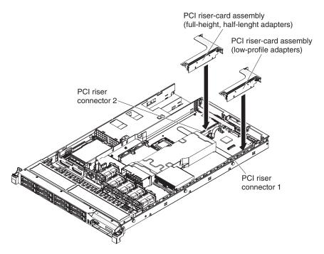
Figure 41. PCI riser-card assembly installation
