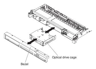
Figure 72. Optical drive cage installation
