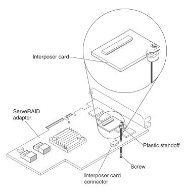
Figure 65. Interposer card installation
