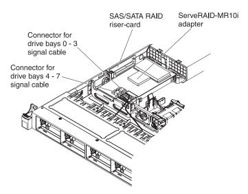
Figure 49. ServeRAID-M10i adapter cable connection
