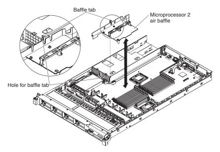
Figure 28. Microprocessor 2 air baffle removal
