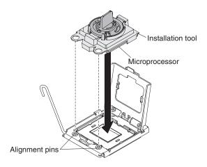
Figure 81. Microprocessor installation
