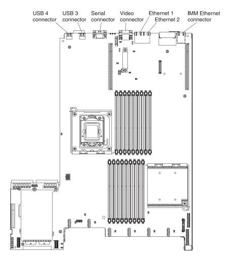
Figure 16. System-board external connectors
