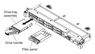
Figure 33. Hot-swap hard disk drive installation
