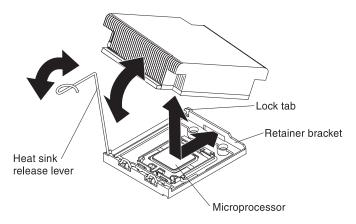
Figure 84. Heat sink installation
