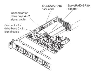
Figure 47. ServeRAID-BR10i adapter cable connection
