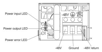
Figure 11. DC power supply LEDs
