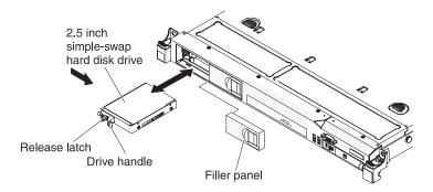
Figure 35. Simple-swap hard disk drive installation
