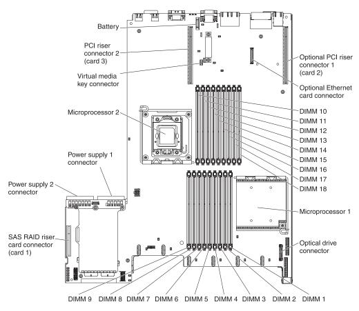
Figure 19. System-board optional device connectors
