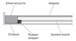
Figure 62. Adapter installation
