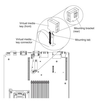
Figure 57. Virtual media key installation
