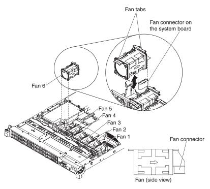
Figure 52. Fan installation
