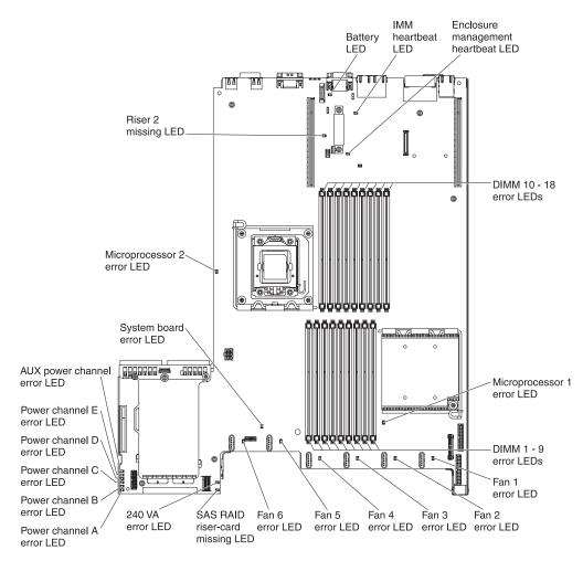
Figure 18. System-board LEDs
