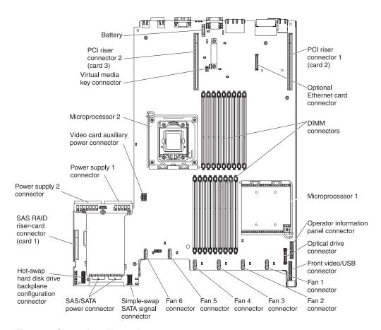
Figure 15. System-board internal connectors
