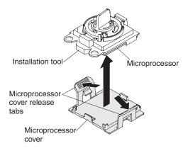
Figure 80. Microprocessor cover removal
