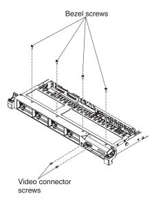
Figure 75. Screws removal
