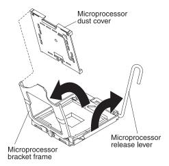
Figure 78. Dust cover removal
