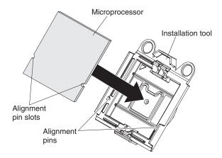
Figure 79. Microprocessor alignment
