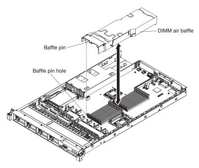
Figure 88. DIMM air baffle installation
