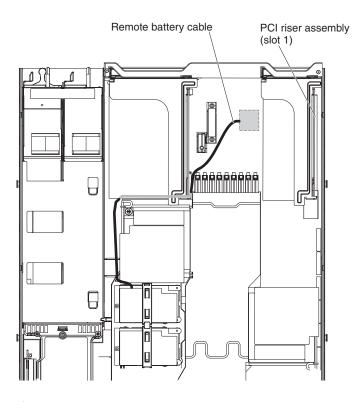
Figure 68. Cable connection
