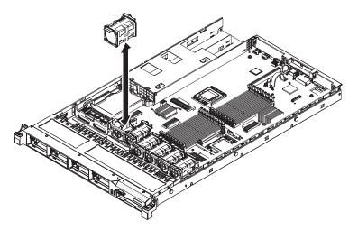
Figure 53. Fan installation
