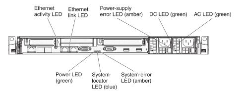
Figure 10. Rear view LEDs
