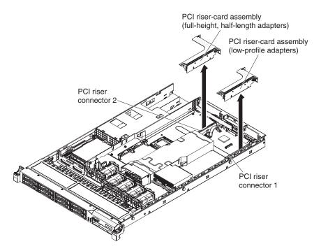
Figure 40. PCI riser-card assembly removal
