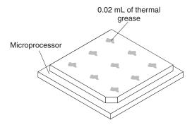
Figure 85. Thermal grease distribution
