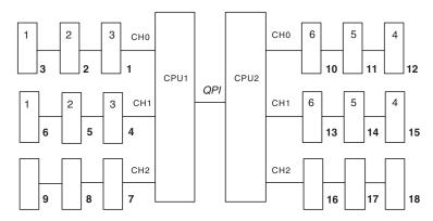
Figure 30. Memory channel interface layout
