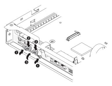
Figure 60. Metal clip installation
