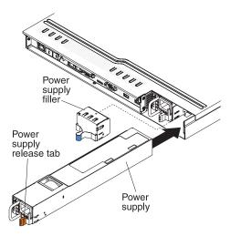
Figure 54. Power supply installation
