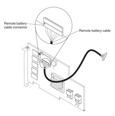
Figure 66. Cable connection
