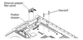
Figure 59. Filler panel removal
