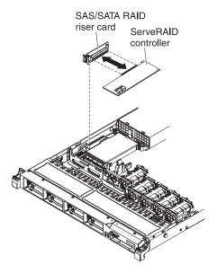
Figure 44. ServeRAID controller installation
