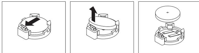
Figure 21. Battery removal
