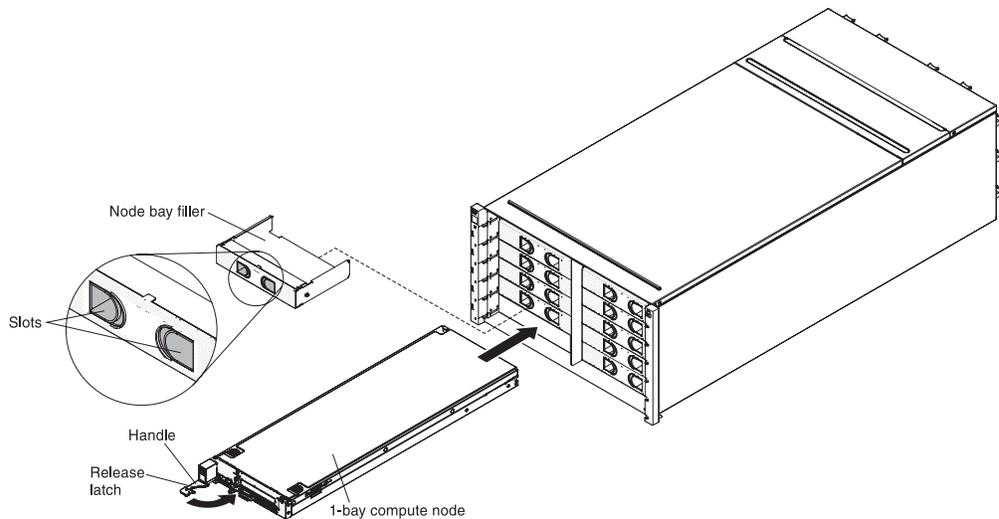
Figure 15. Installation of a 1-bay compute node
