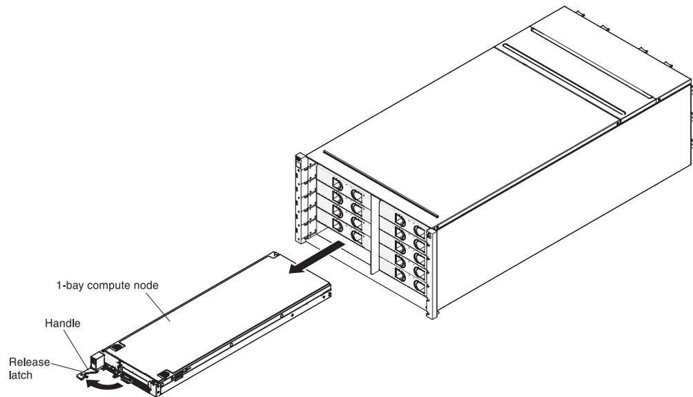
Figure 14. Removal of a 1-bay compute node
