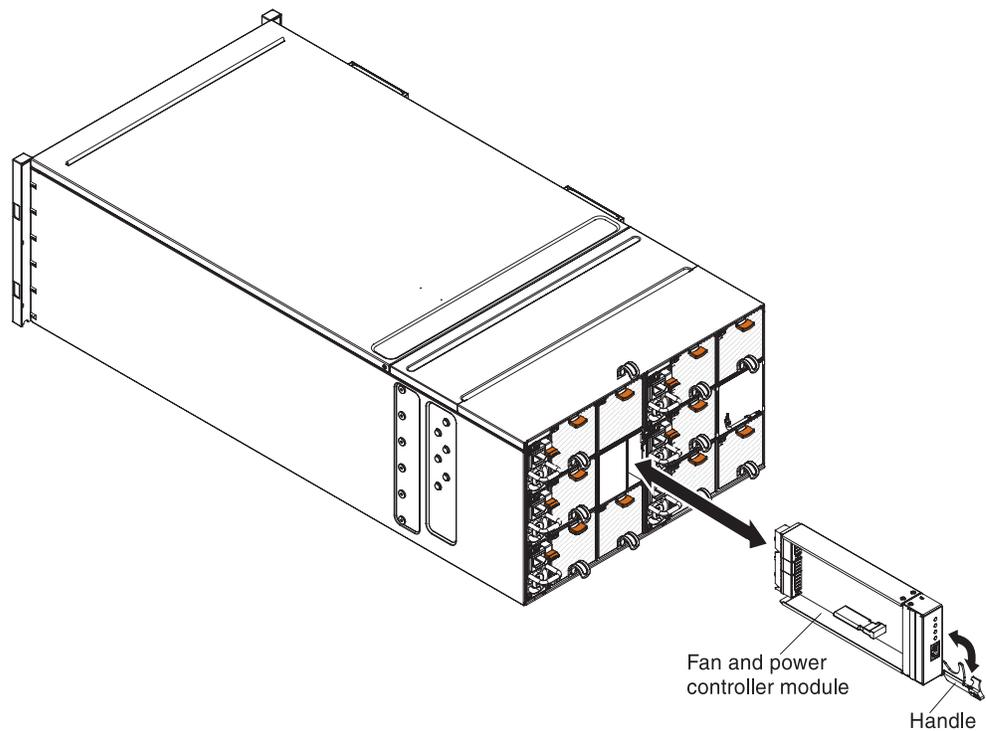
Figure 18. Removal of a fan and power assembly from the chassis
