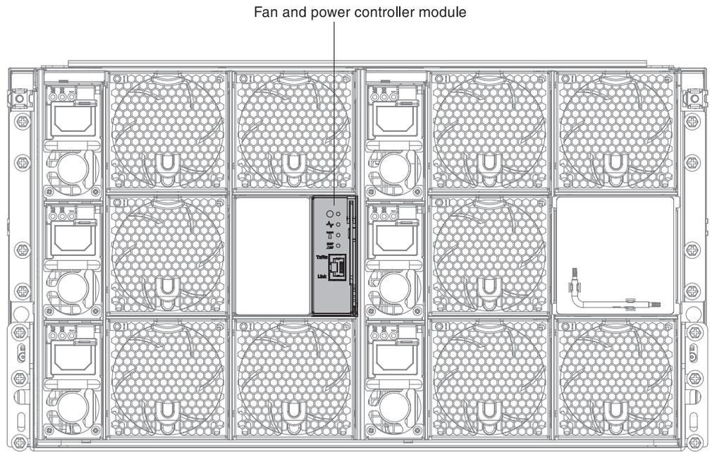
Figure 8. Chassis fan and power controller bay
