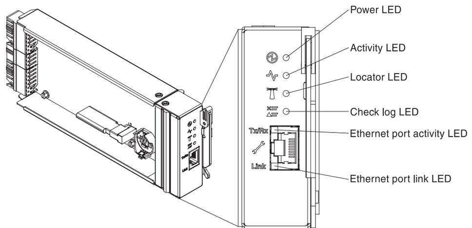
Figure 9. Fan and power controller with call outs
