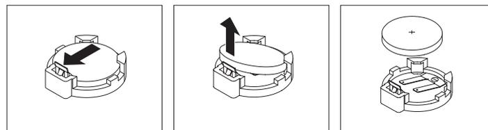
Figure 23. Battery removal
