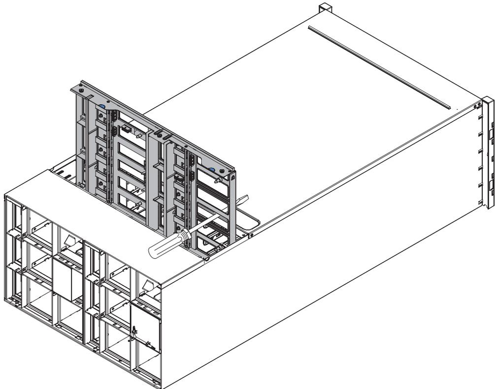
Figure 30. Removal of the chassis midplane from a chassis
