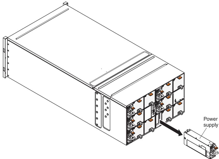
Figure 27. Removal of a power supply
