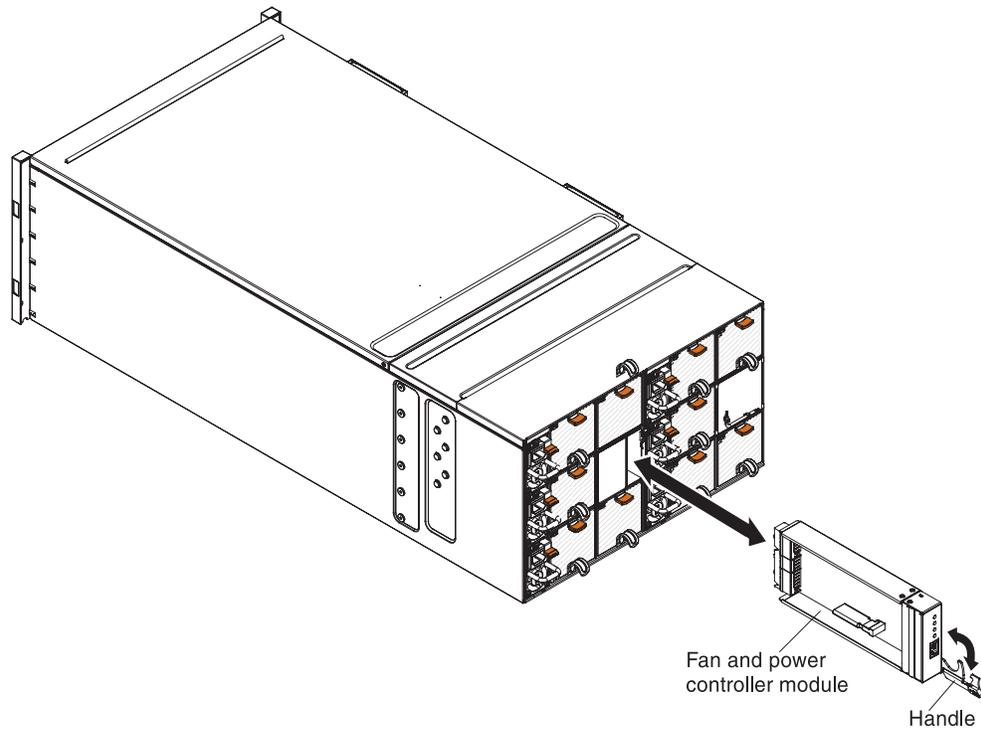
Figure 19. Installation of a fan and power controller into the chassis
