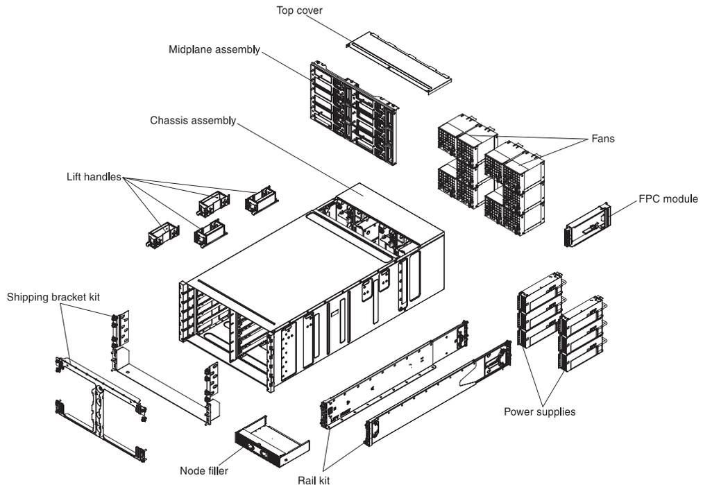
Figure 4. Chassis components
