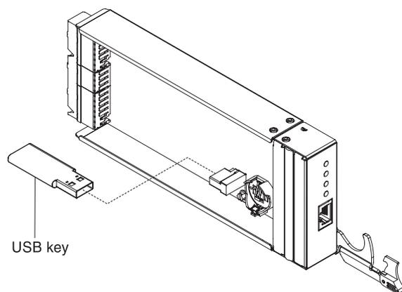
Figure 25. USB flash drive removal
