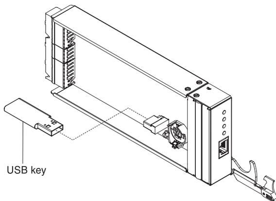
Figure 26. Installing USB flash drive
