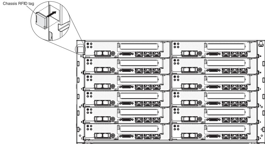
Figure 2. The location of the Chassis RFID tag
