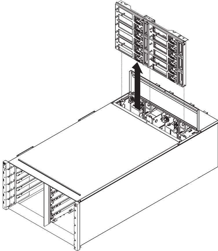
*Figure 31. Removal of the chassis midplane from a chassis*
