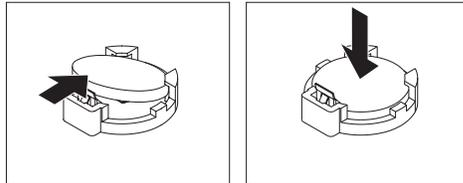
Figure 24. Battery installation
