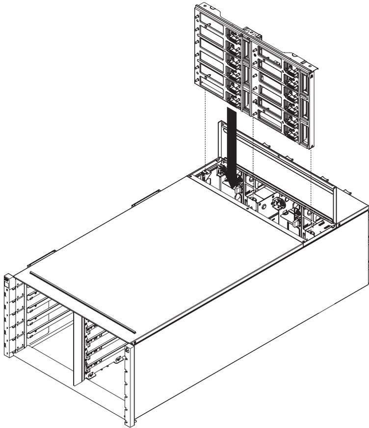
*Figure 32. Installation of a chassis midplane into a chassis*
