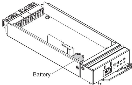
Figure 20. Locate the battery
