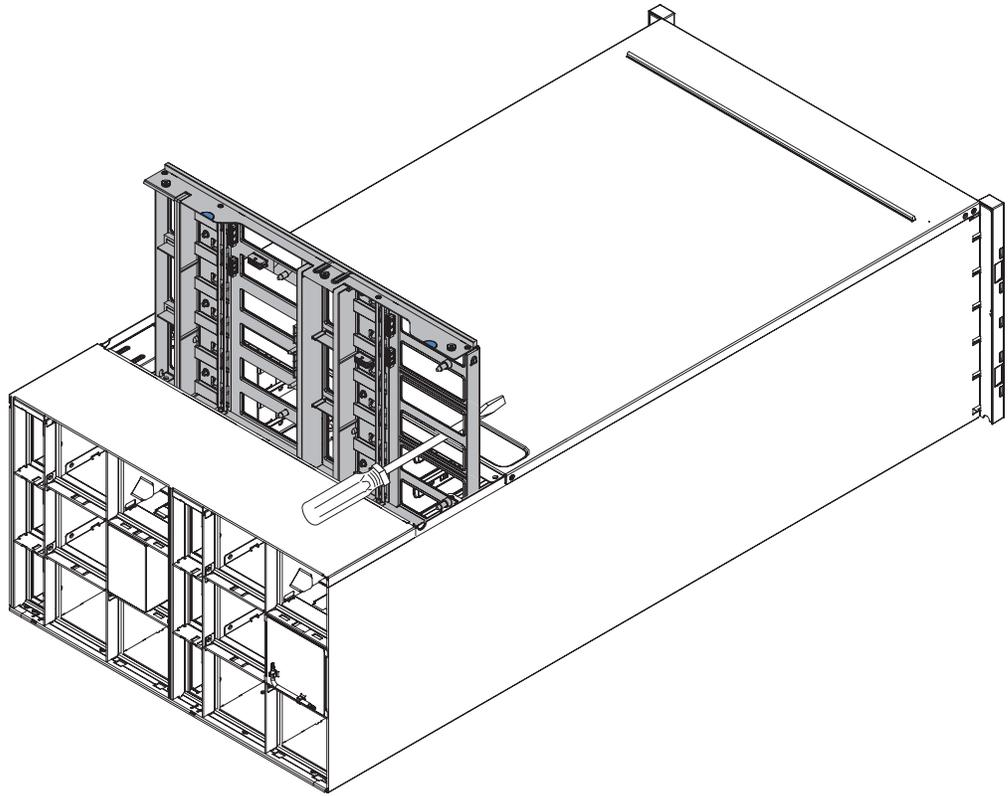
Figure 33. Installation of a chassis midplane into a chassis
