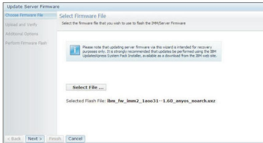
6. Click **Next >** to begin the upload and verify process on the selected file. A progress meter will be displayed as the file is being uploaded and verified (as shown in the following illustration).
