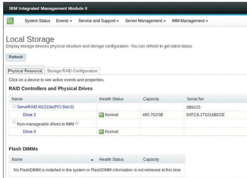
Click the link of the supported RAID controller to view the controller's active events, hardware, firmware, and port information.
