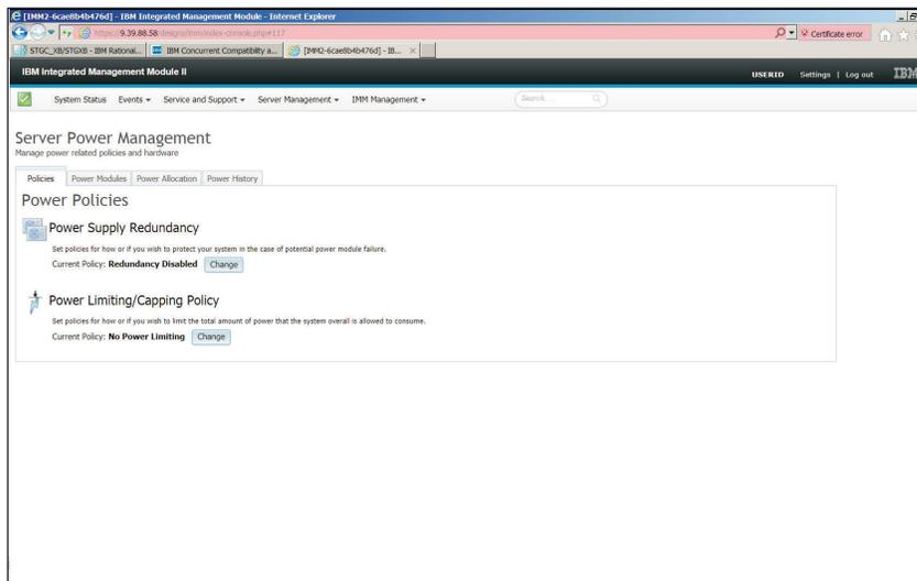
To select the policy you want to use to protect the server in the case of a potential power module failure, click the Current Policy **Change** button for the Power Supply Redundancy option on the Power Policies window. You will see a window similar to the following illustration. By choosing a power policy you can trade off between redundancy and available power.
