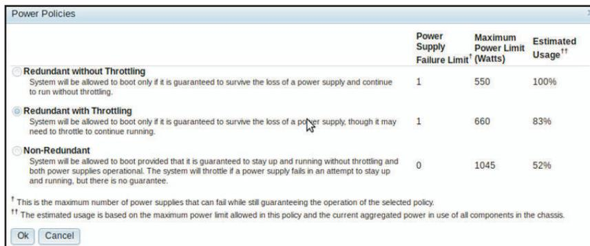
With Active Energy Manager you can limit the total amount of power that the server is allowed to use. To set a limit for server power usage, click the Current Policy **Change** button for the Power Limiting/Capping Policy option on the Power Policies window.
