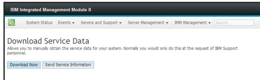
The process of collecting the service and support data starts. This process takes a few minutes to generate the service data that you can save to a file.
