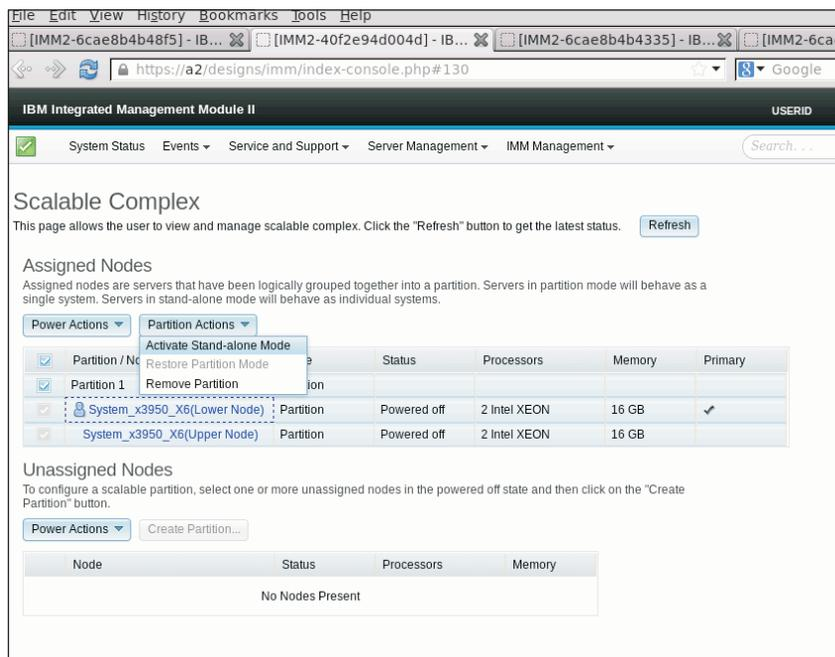
Click **Activate Stand-alone Mode** to allow each node to act independently of one another. Click **Restore Partition Mode** to switch between the partition and stand-alone modes. Click **Remove Partition** to remove the partition.
