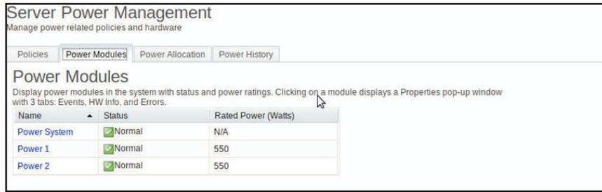
The following illustration shows the **Power Modules** tab for servers that can support up to four power supplies.
