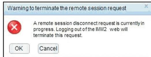
After the remote control user receives the request, the user must determine whether to release the remote session in the interval time selected before starting the remote control session. A Request to End Remote Session window is displayed to remind the remote control user of any time remaining. The Request to End Remote Session window is shown in the following illustration.
