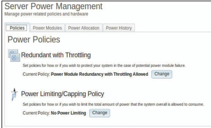
To select the policy you want to use to protect your server in the case of a potential power module failure, click the Current Policy **Change** button for the Redundant with Throttling option on the Power Policies window.
