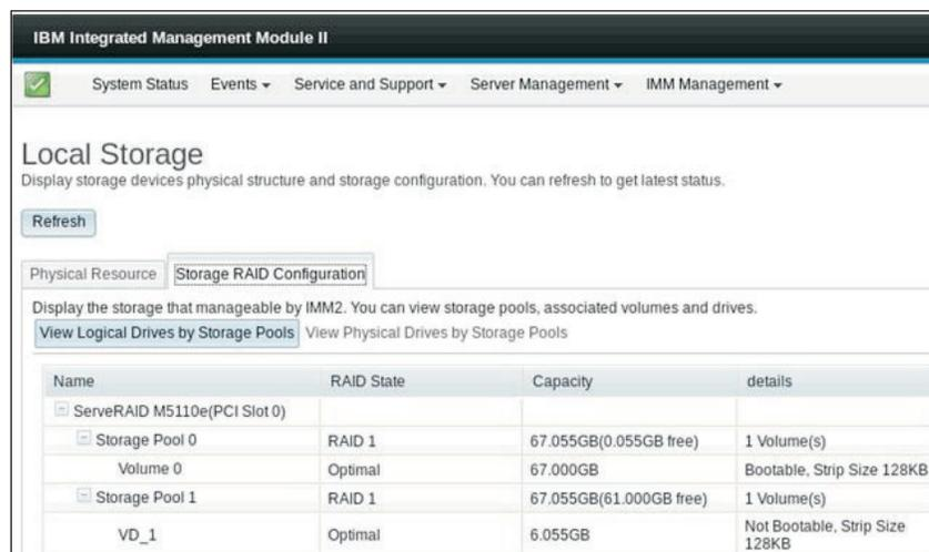
To view the physical drives and associated storage pools click the **View Physical drives by Storage Pools** tab (as shown in the following illustration). The capacity and RAID level of the storage pool is displayed. The RAID state of the drive, the number of drives in the storage pool, along with the interface and one drive type are displayed.
