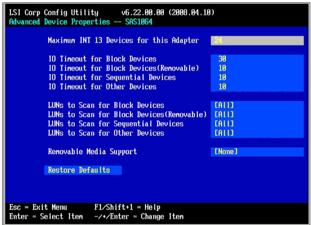
Figure 152. Setting for Block Device Timeouts
