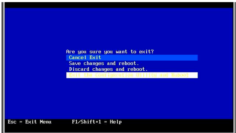
Figure 159. Saving the BIOS setting and rebooting
