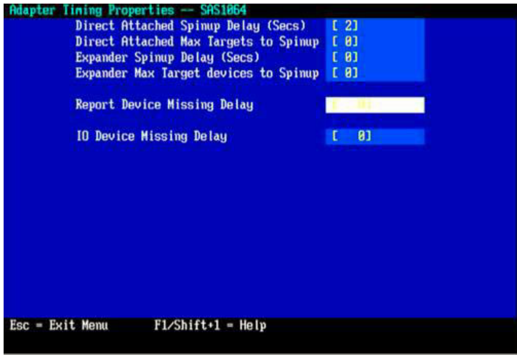
Figure 158. SAS Adapter timing properties for VMware
