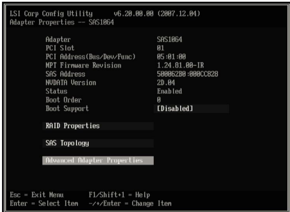
Figure 61. Disabling boot support for the SAS Expansion Card
