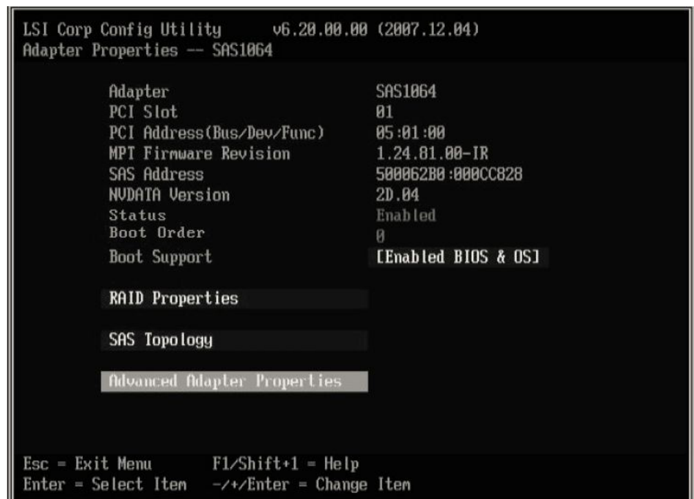
Figure 67. Adapter Properties screen showing enabled BIOS and OS boot support
