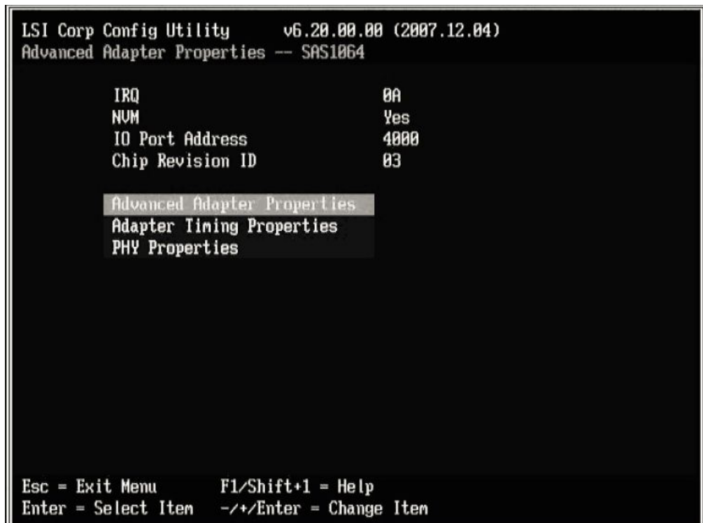
Figure 68. Advanced Adapter Properties screen
