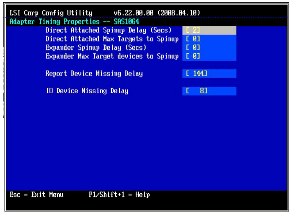
Figure 156. SAS 1064 Adapter timing properties for Windows
