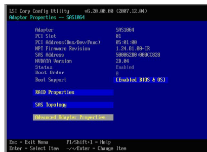
Figure 11. Adapter Properties screen showing enabled BIOS and OS boot support for the SAS Expansion Card
